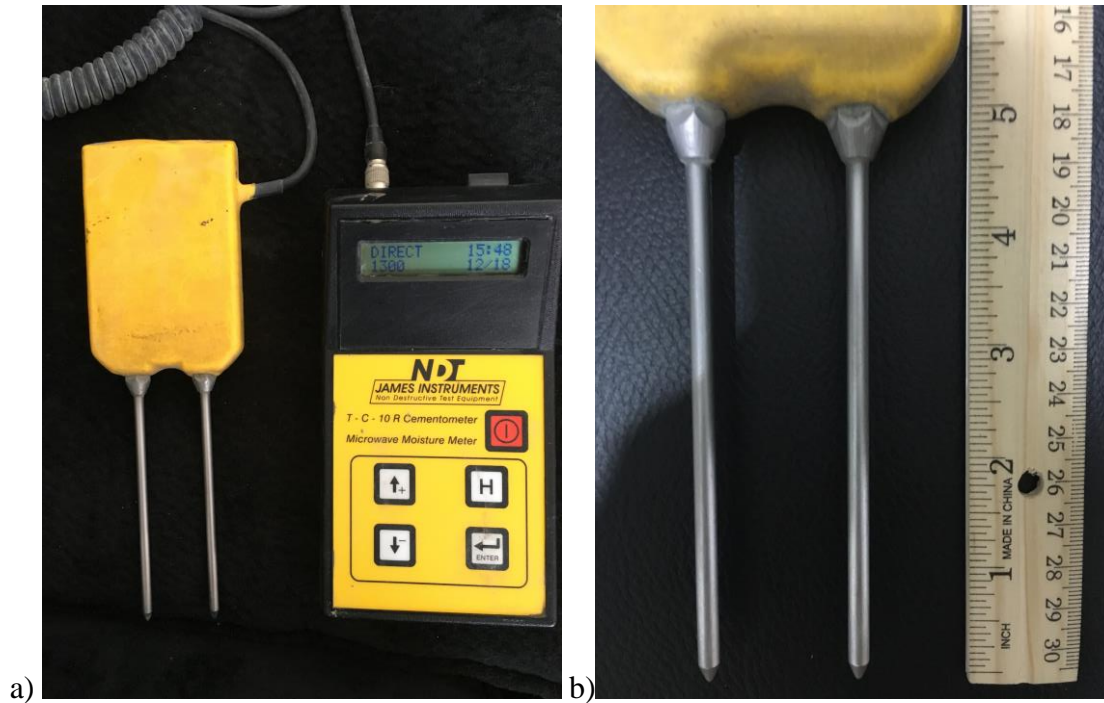
Figure 2.5 a) Cementometer™ probe device and handheld device; and b) probes with a ruler for scale.
