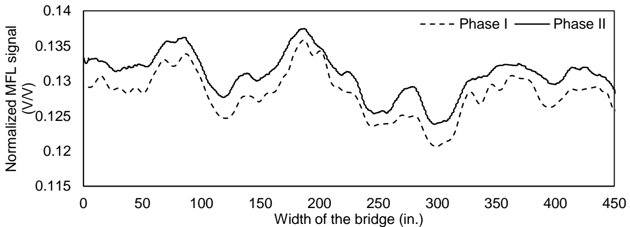
Figure 5-8: Comparison of MFL signal from phase I and phase II on span 1 tendon 2.
