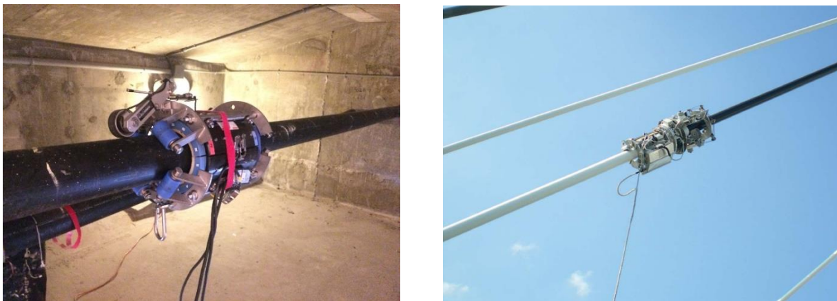
Figure 1-3: MFL of an external PT tendon (Lau and Azizinamini, 2018) and cable stays (Alpin Technik Leipzig accessed online 2020).
