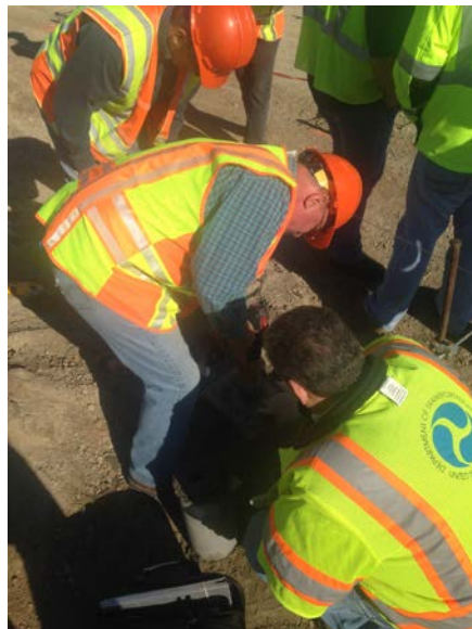
Figure 26: AVA sample being taken from a standard beam mold
