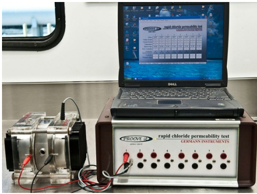
Figure 30: Rapid Chloride Permeability Test
