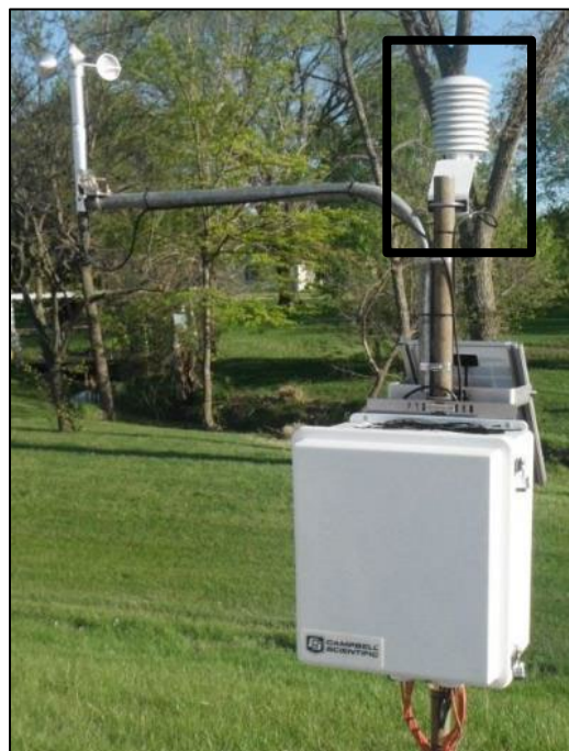
Figure 2.4: Rotronic HygroClip2 Temperature/Relative Humidity Probe Inside Solar Radiation Shield (outlined by black rectangle) Attached to Data Logging Equipment
