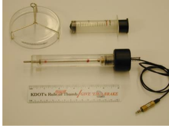
Figure 3 Petri dish, 20 ml syringe, and temperature sensor
