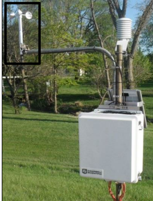
Figure 2.3: Met-One Anemometer (outlined by black rectangle) Attached to Data Logging Equipment
