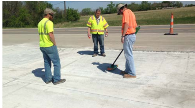
Figure 41: KDOT staff measuring Pavement Thickness using the MIT Scan T2
