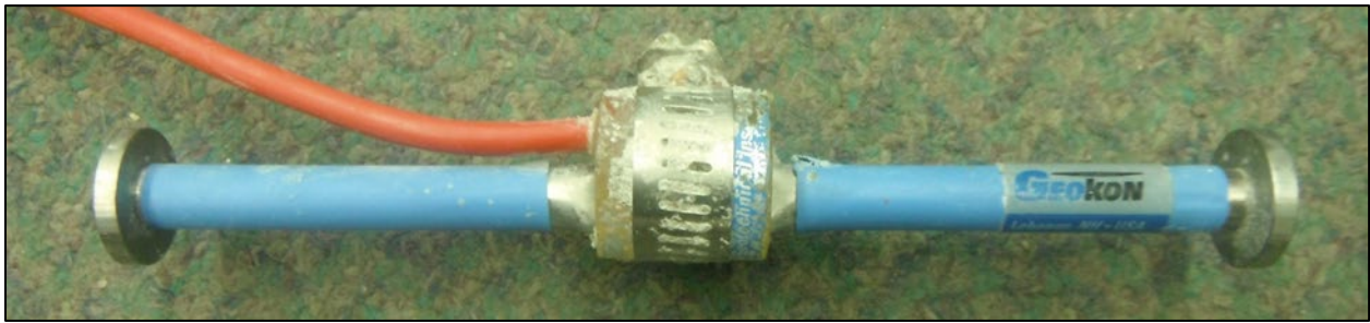
Figure 2.1: Geokon 4200 Vibrating Wire Strain Gage
