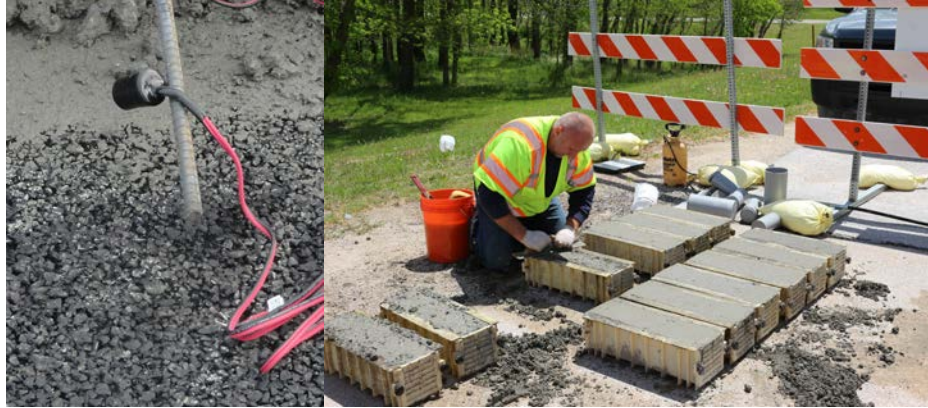
Figure 21 (a): Maturity Logger Figure 21(b): Beams for the Maturity Curve
