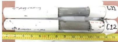
Figure A3. Neat grout test specimens for PTI after 28-day and 56-day hydration
