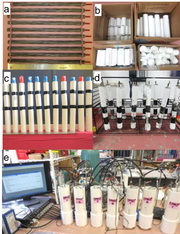
Figure 2.1. PTI Accelerated Corrosion Testing
