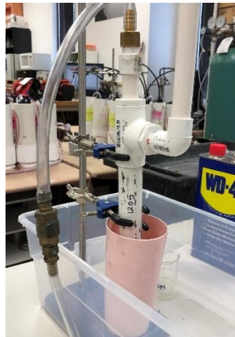
Figure 2.4. Photo of injection port.
