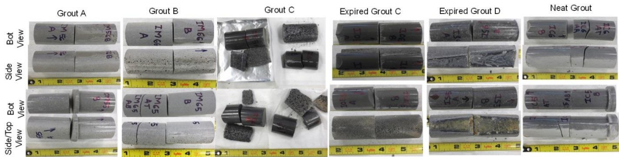
Figure A8. INT Tee-body test specimen after opening, cast with extra 10% mix water
