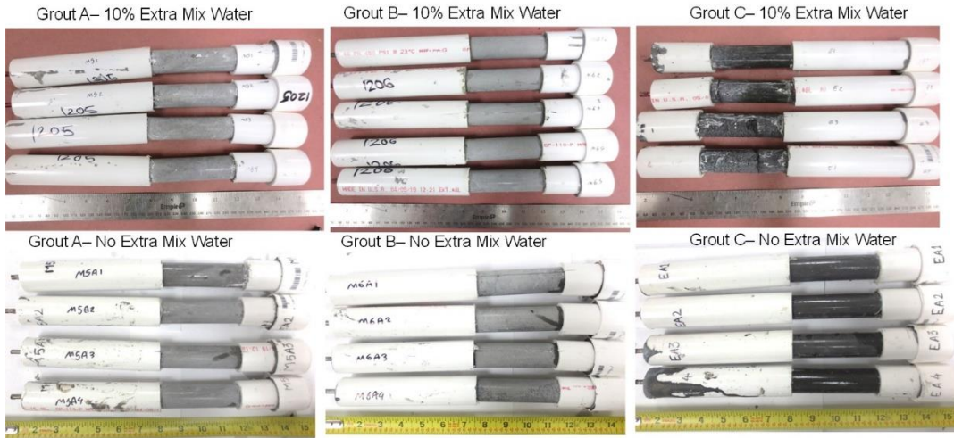
Figure A1. PTI test specimens after 28-day hydration (Top: with 10% excess mix water, Bottom: with no 10% excess mix water)
