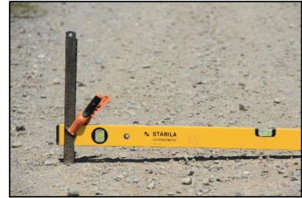
Figure 3.8: Bubble level for measuring crown and rut depth.
