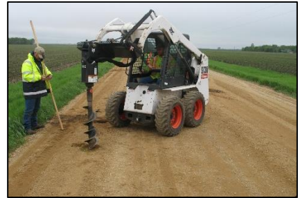
Figure 3.18: Sampling with a mechanical augur.
