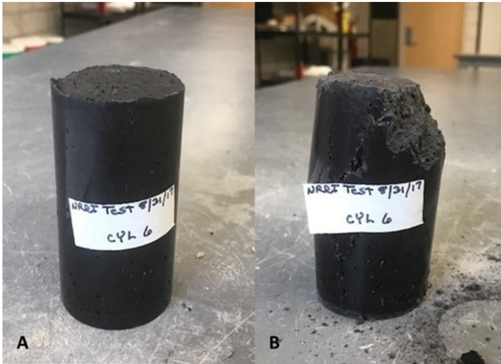
Figure 2.20 2" x 4" test cylinders, before (A) and after (B) uniaxial compressive strength testing.
