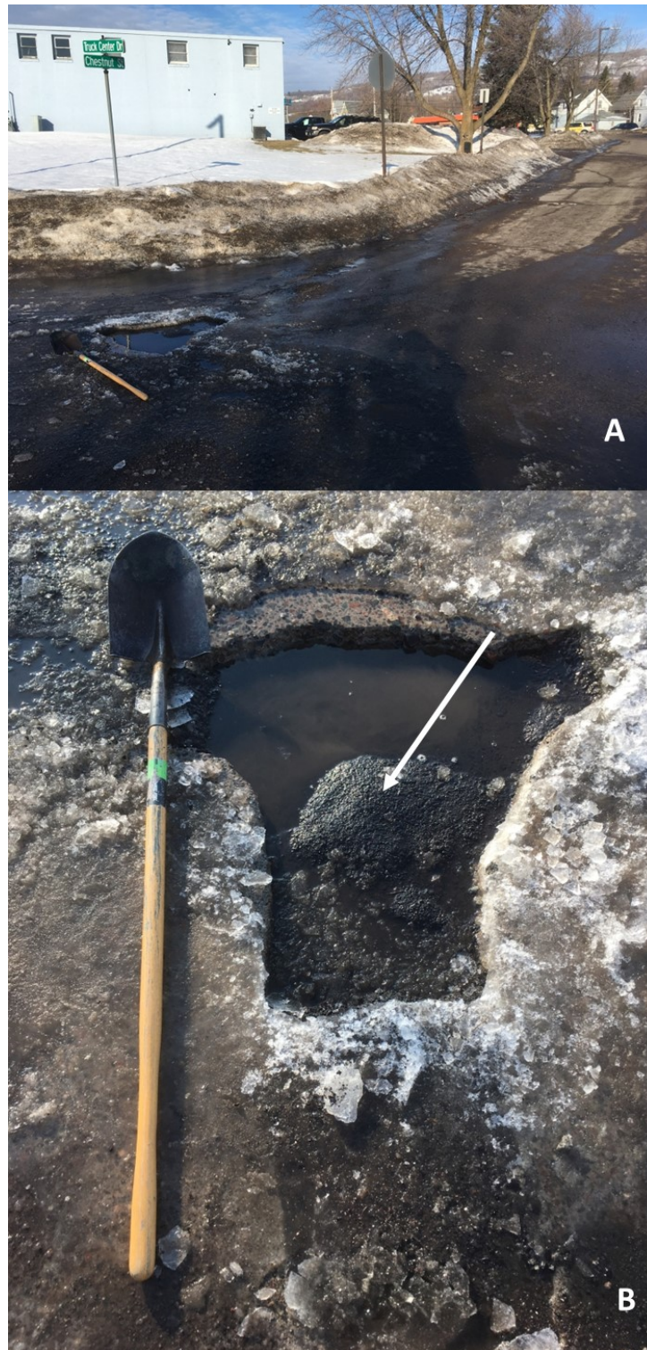
Figure 2.77 Site conditions (A); and resistant remnant of June 7, 2018, Duluth field trial repair (B); as of March 19, 2019.
