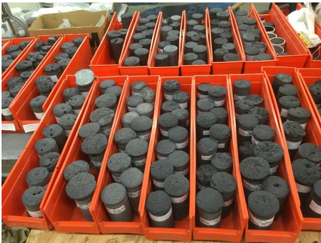
Figure 2.37 Some of the 2" diameter x 4" tall cylinder specimens prepared during formulation development.
