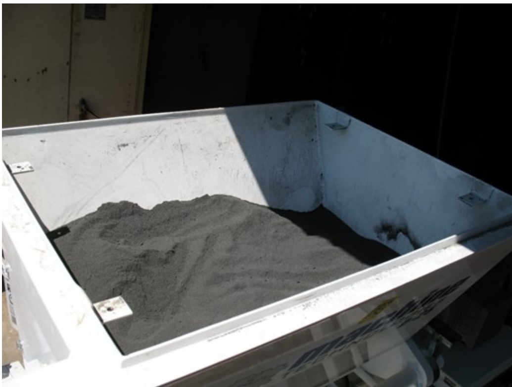
Figure 2.18 Continuous mixer hopper filled with reactive aggregate.
