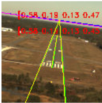
Figure 21: Prediction (top numbers) and ground truth (bottom numbers) of the 6 runway image parameters.
