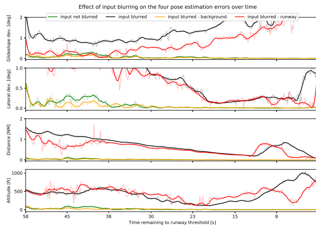
Figure 46: Global saliency for a single approach from the Florida X59-10 dataset. The expectations with regards to the four input types depicted in Figure 40 can be confirmed. In nearly all cases, the prediction error on input where the runway is blurred is significantly higher than the error on input where the background is blurred. A region of interest for further examination is the [58, 38] second interval on the glideslope deviation error graph.
