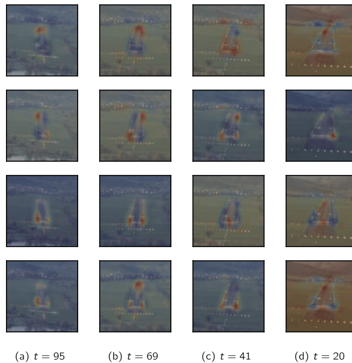
Figure 43: Local saliency heatmaps for a single approach from the Buochs dataset. The time remaining t towards the runway threshold is shown from left to right. The four pose parameters, from top to bottom, are the glideslope deviation error, the lateral deviation error, the distance error, and finally the altitude error. Red areas indicate a higher relative importance on the predicted pose compared to the blue areas. This particular heatmap shows that as the runway comes closer, there is less importance on the runway corners (especially for glideslope, distance and altitude estimates) and more importance towards its surroundings.
