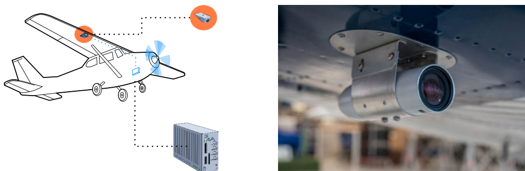
Figure 3: Left: Illustration of the VLS (forward-looking camera and compute box). Right: Camera mounted on an aircraft during flight testing.
