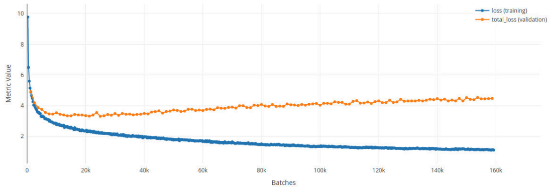
Figure 33: Evolution of the loss on the training and validation sets for the first experiment, as a function of processed batches of data. One batch of data represents a given number of training samples. This displays overfitting.
