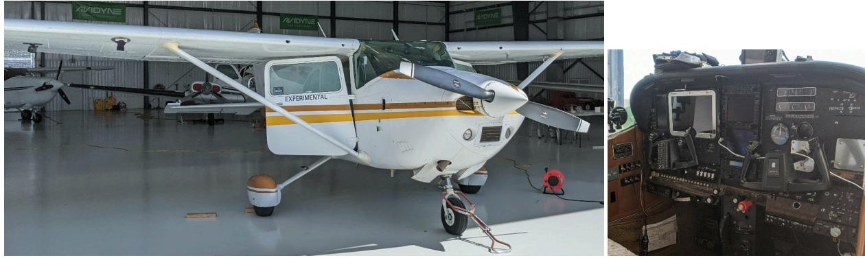
Figure 15: Experimental Cessna C182 with forward facing camera mounted under the right wing and additional tablet display in the cabin.
