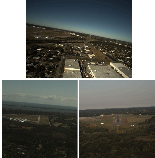
Figure 26: Various runway locations: multiple, visual and precision instrument runways, anticlockwise from the top.
