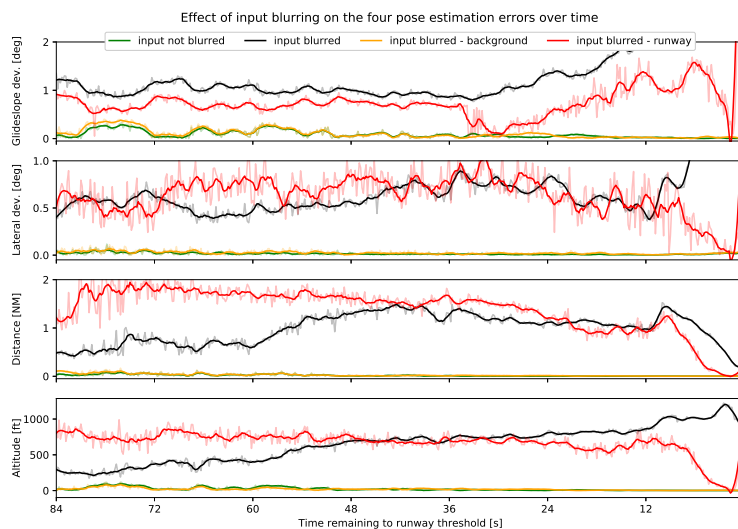
Figure 42: Global saliency for a single approach from the Brno dataset. The expectations with regards to the four input types depicted in Figure 40 can be confirmed. In almost all cases, the prediction error on input where the runway is blurred is significantly higher than the error on input where the background is blurred. A region of interest for further examination is the [34, 26] second interval on the glideslope deviation error graph.
