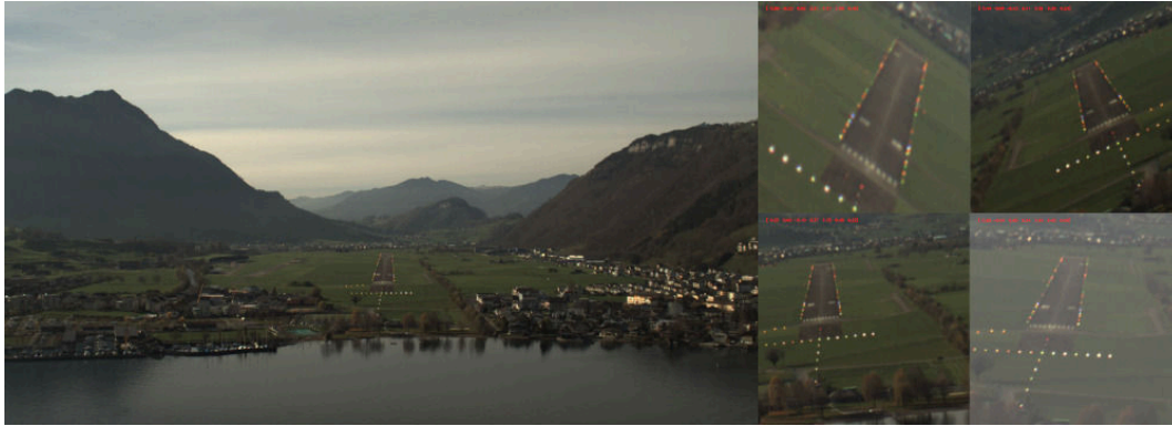
Figure 32: Original image and generated training data for the Runway extractor network after cropping and augmentations.
