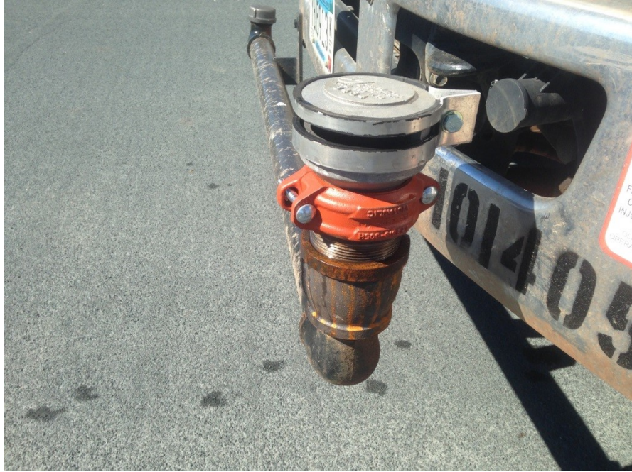
Figure 2.5 United Equipment adjustable water truck nozzle.
