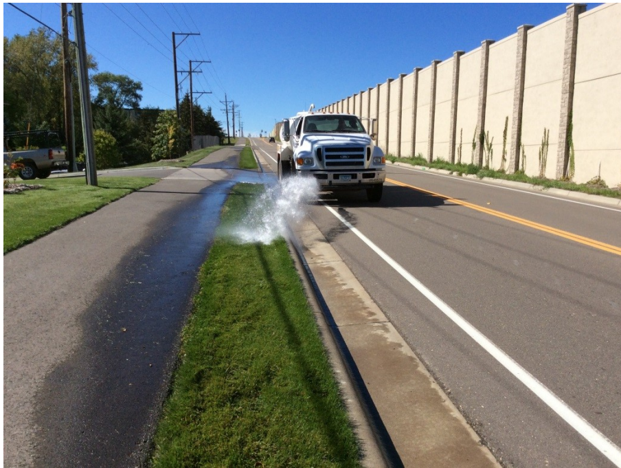
Figure 2.6 An example of a water truck nozzle with a tight pattern.
