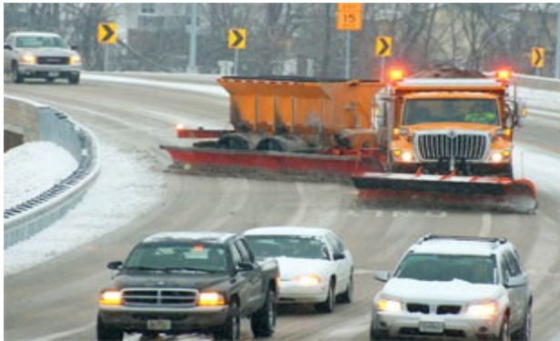
Figure 1.3: Tow Plow in operation
