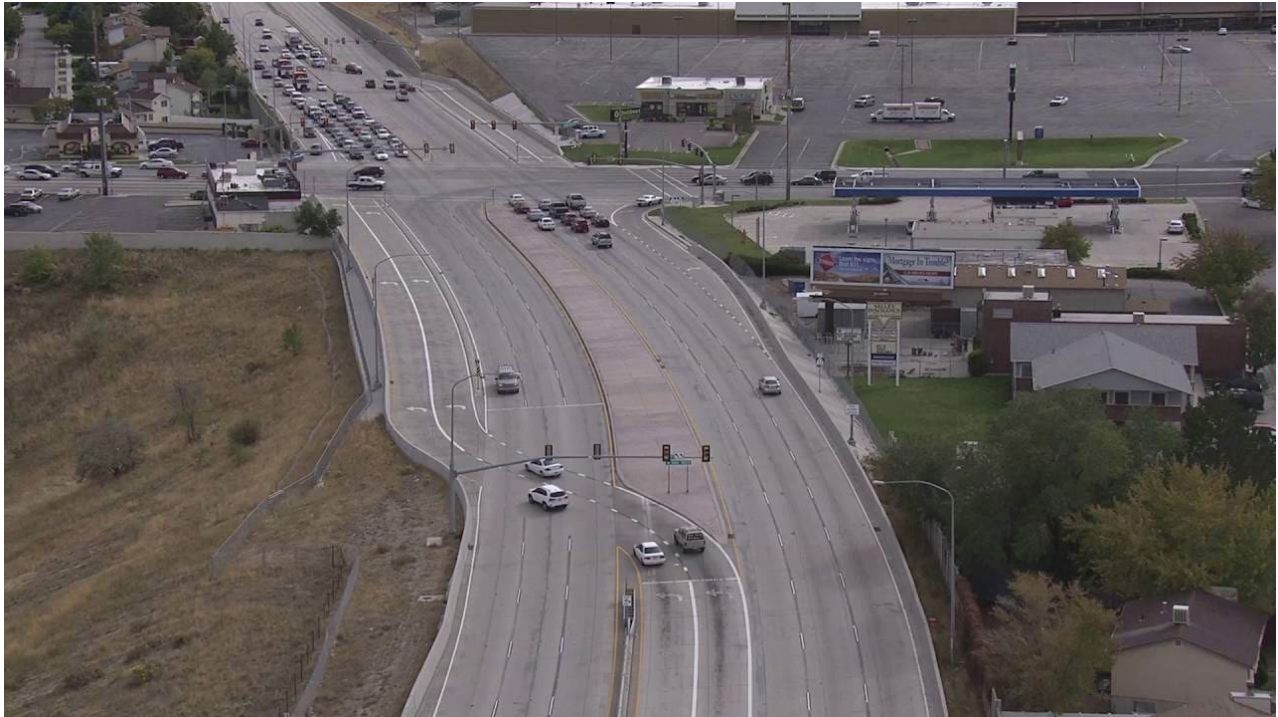
Figure 4.1: Displaced left-turn intersection
