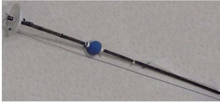
FIGURE 3 Fabrication of a Void Specimen, with a Rubber Ball Used to Simulate a Void.
