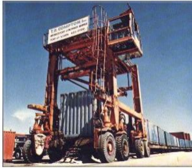
Container-on-flat-car (COFC) with gantry crane at intermodal yard
