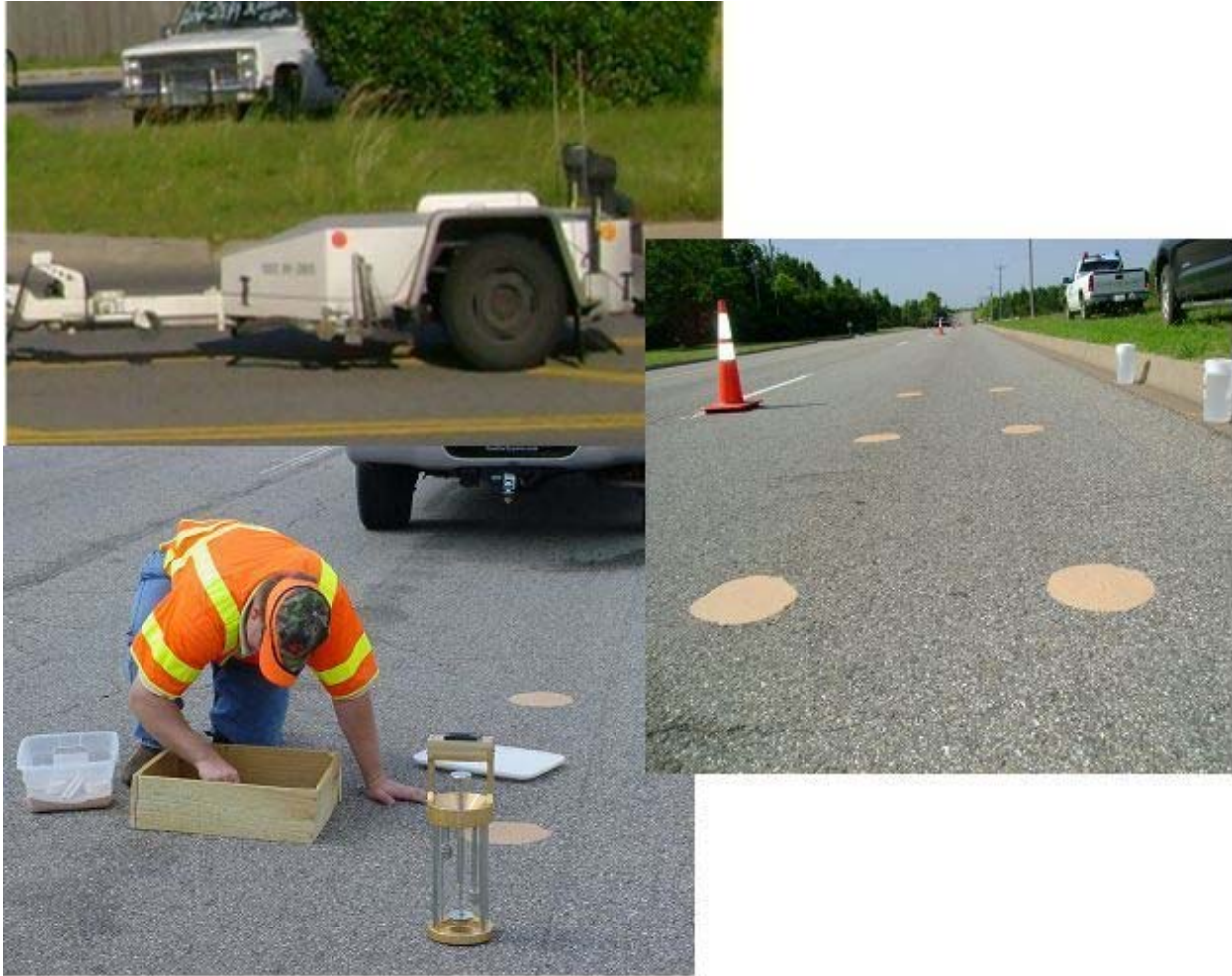
Figure 5: (Clockwise from the top) ODOT Skid Tester, Sand Circle Tests, and Outflow Meter/Sand Circle Testing in Progress
