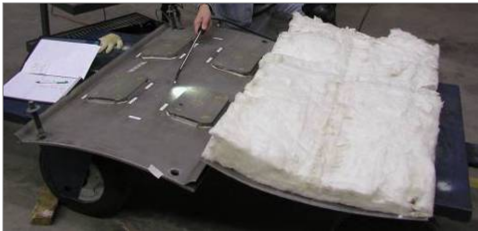
Figure 21. Tank Car Fillet Weld Test Panel with Cover and Hinged
