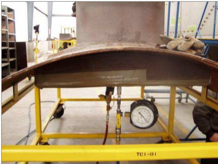
Figure 49. Leak Test Master Gage Test Specimen Showing Air Hose Connection and Pressure Gage
