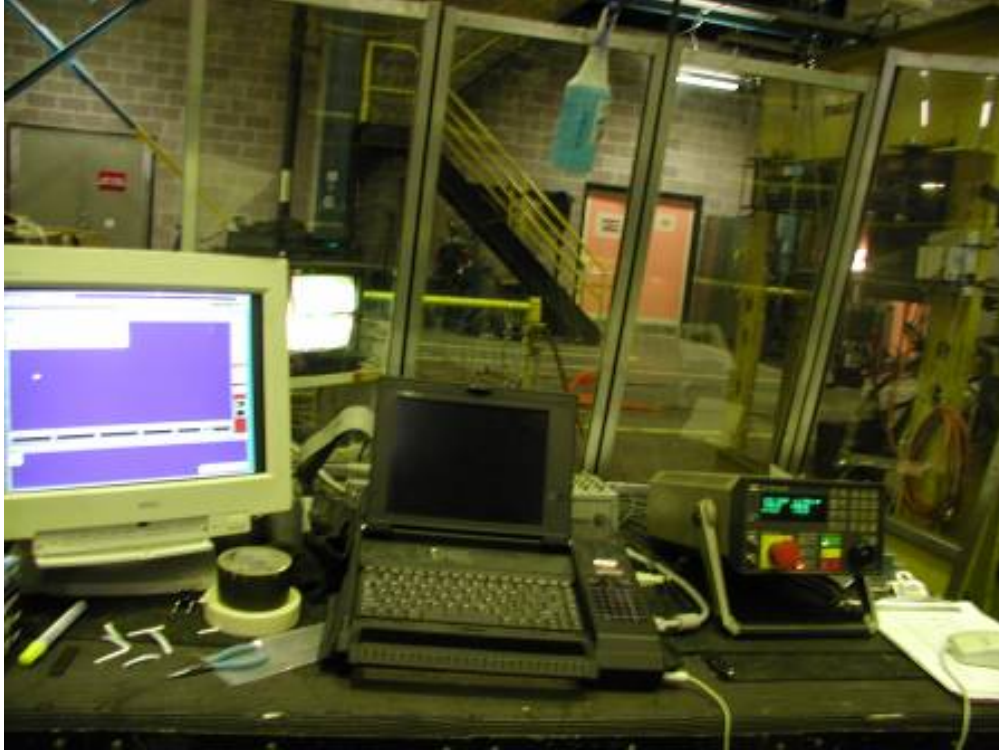
Figure 16. Instrumentation Used in the Setup for Tank Car Test Panel Dynamic Loading
