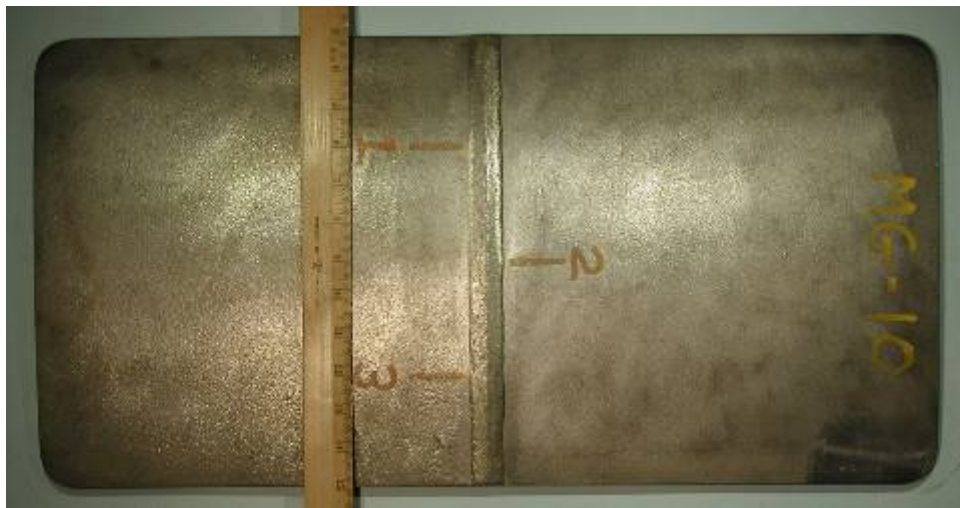
Figure 26. Tank Car Butt Weld Master Gage with Fatigue Cracks at Weld Toe
