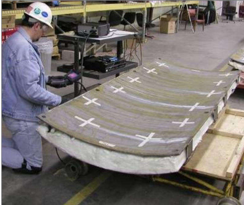
Figure 22. Tank Car Fillet Weld Test Panel Undergoing Remote Visual Inspection
