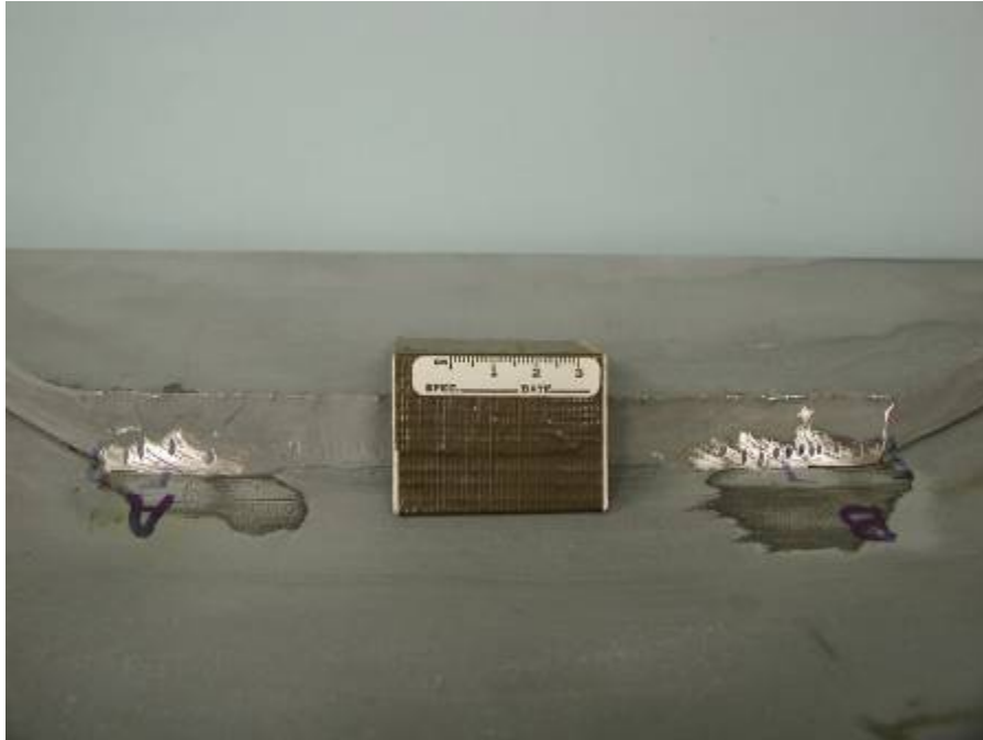
Figure 23. Tank Car Fillet Weld Master Gage with EDM Notches at Weld Terminations
