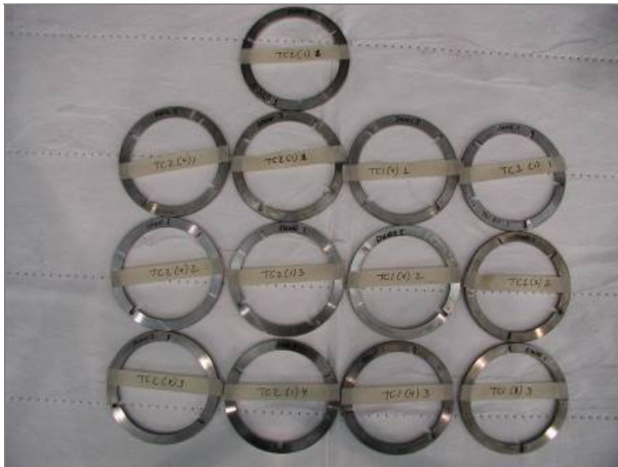
Figure 44. Several Samples with Different Known Leak Path Sizes
