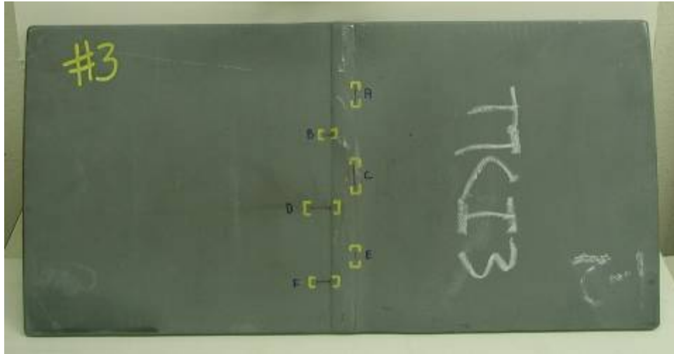
Figure 25. Tank Car Butt Weld Master Gage with EDM Notches at Weld Toe
