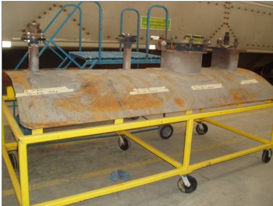
Figure 46. Tank Car (Leak Test Mock-Up) Section Containing Multiple Ports
