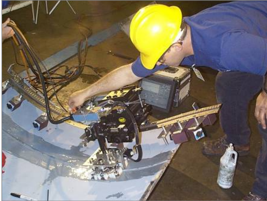
Figure 4. AUT Setup on Butt Weld Test Panel at TTC
