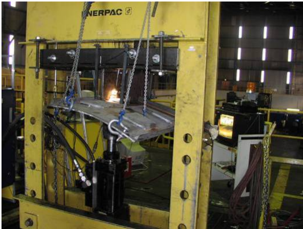
Figure 17. Tank Car Test Panel Setup for Dynamic Loading on the 200,000-Pound Load Frame
