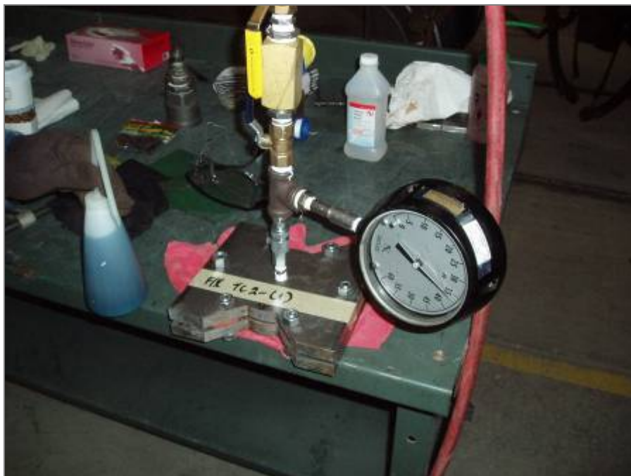
Figure 47. Leak Test Master Gage Test Specimen
