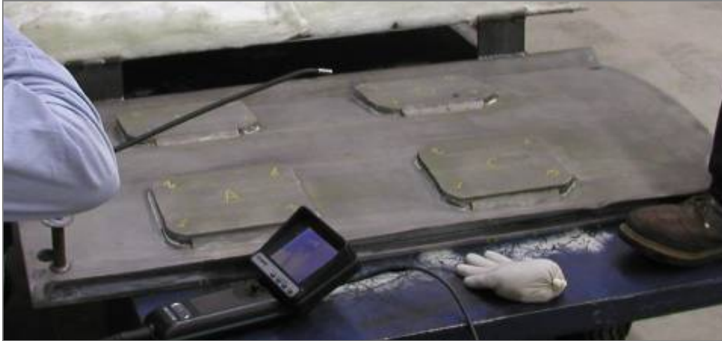
Figure 20. Tank Car Fillet Weld Test Panel
