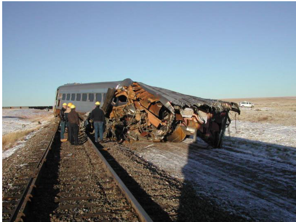
Figure 7. Cab-Car after Impact
