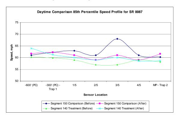
Figure D-11. Daytime Comparison 85<sup>th</sup> Percentile Speed Profile for SR 87.
