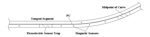
Figure 4. Equipment Layout at Each Data Collection Site (Left Curve).
