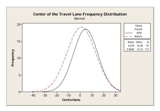
Figure C-2. Frequency Distribution of Lateral Vehicle Position at SR 14 (Right) Curve Location.
