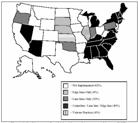
Figure A-1 – Line types for which wider markings are used in state DOTs.
