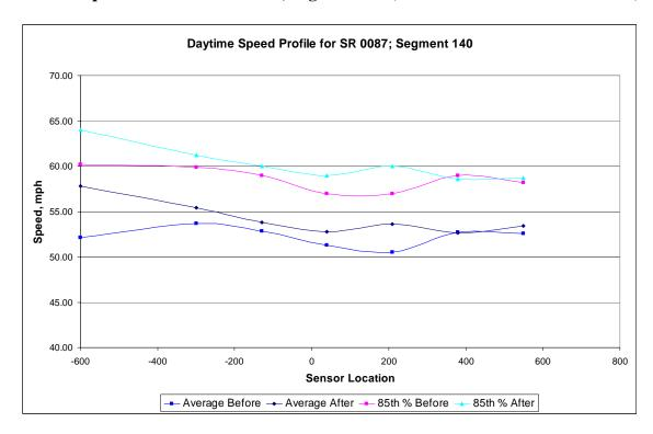
Figure D-7. Daytime Speed Profile for SR 87, Segment 140 (Treatment Site).
