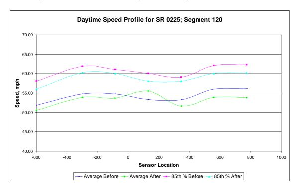
Figure D-17. Daytime Speed Profile for SR 225, Segment 120 (Treatment Site).
