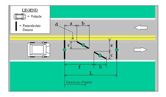
Figure 5. Geometric Layout of Piezoelectric Sensors (48).
