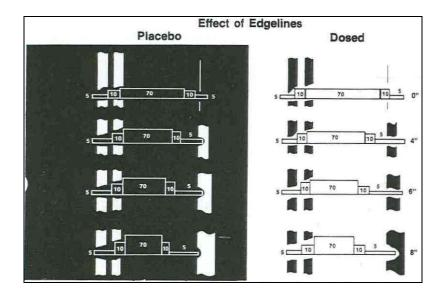
Figure 2. Driver Path Range: Effect of Edge Lines (42).
