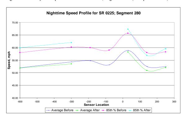
Figure D-20. Nighttime Speed Profile for SR 225, Segment 280 (Comparison Site).
