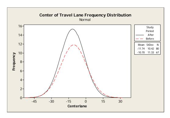
Figure C-4. Frequency Distribution of Lateral Vehicle Position at SR 87 (Left) Curve Location.
