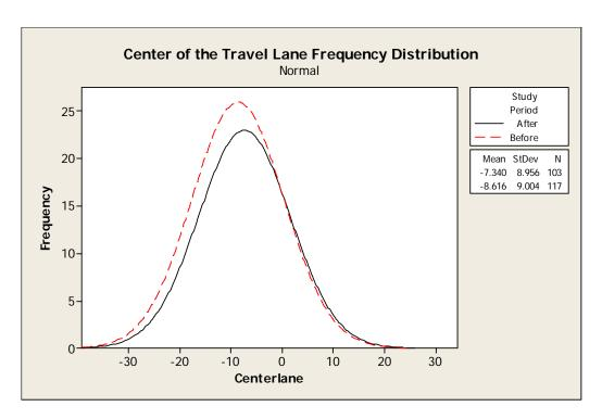
Figure C-1. Frequency Distribution of Lateral Vehicle Position at SR 14 Tangent Location.
