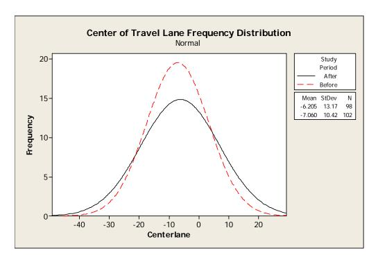
Figure C-6. Frequency Distribution of Lateral Vehicle Position at SR 118 (Left) Curve Location.
