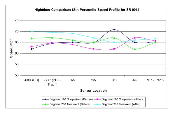
Figure D-6. Nighttime Comparison 85<sup>th</sup> Percentile Speed Profile for SR 14.
