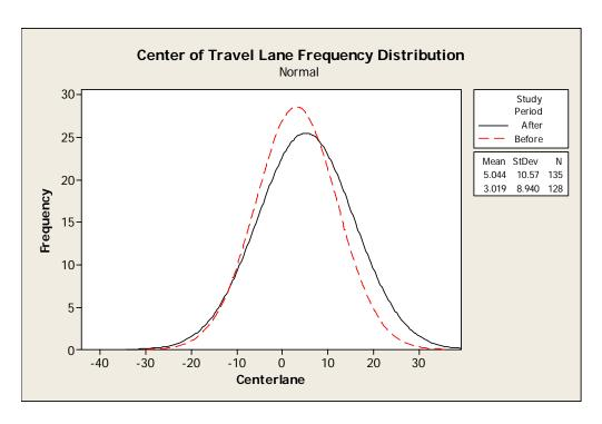
Figure C-8. Frequency Distribution of Lateral Vehicle Position at SR 225 (Right) Curve Location.
