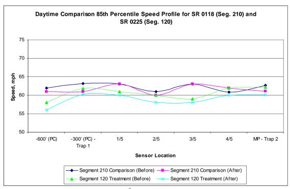
Figure D-21. Daytime Comparison 85<sup>th</sup> Percentile Speed Profile for SR 118, Segment 210 and SR 225, Segment 120.
