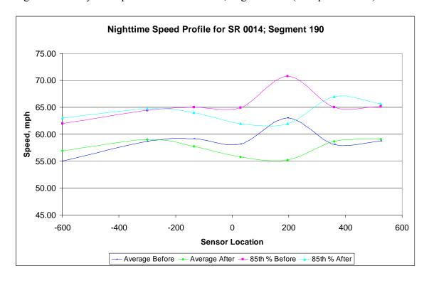
Figure D-2. Nighttime Speed Profile for SR 14, Segment 190 (Comparison Site).
