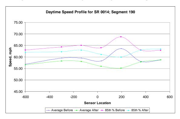
Figure D-1. Daytime Speed Profile for SR 14, Segment 190 (Comparison Site).
