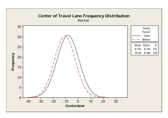
Figure C-7. Frequency Distribution of Lateral Vehicle Position at SR 225 Tangent Location.
