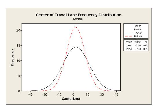
Figure C-5. Frequency Distribution of Lateral Vehicle Position at SR 118 Tangent Location.
