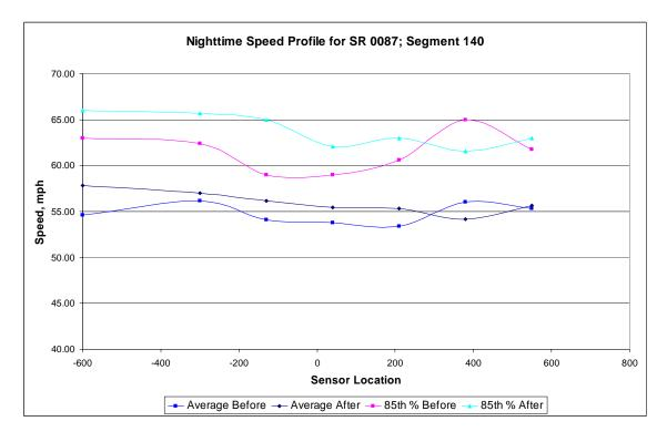
Figure D-8. Nighttime Speed Profile for SR 87, Segment 140 (Treatment Site).
