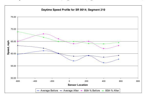
Figure D-3. Daytime Speed Profile for SR 14, Segment 210 (Treatment Site).
