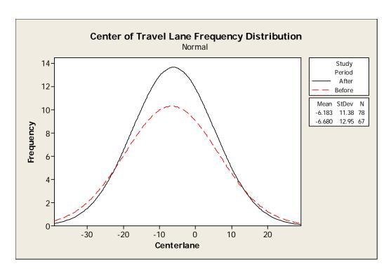
Figure C-3. Frequency Distribution of Lateral Vehicle Position at SR 87 Tangent Location.
