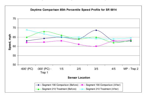
Figure D-5. Daytime Comparison 85<sup>th</sup> Percentile Speed Profile for SR 14.
