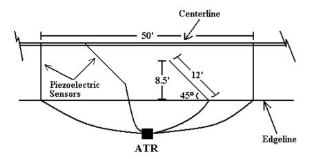
Figure 3. Layout of Sensor Equipment at Trap Location.
