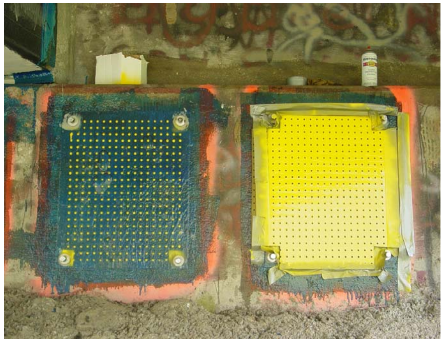
Figure 3.7: Grid marked for measurement at 1" centers.
