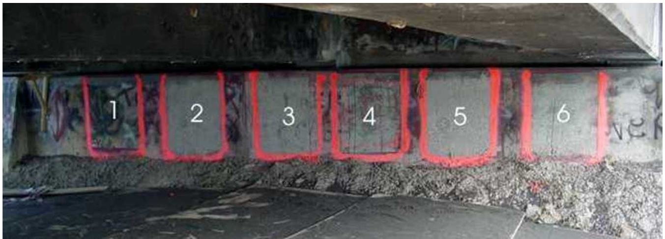
Figure 1.5: Sandblasting for the test panels on the abutment (left) and one of the bents (right).
