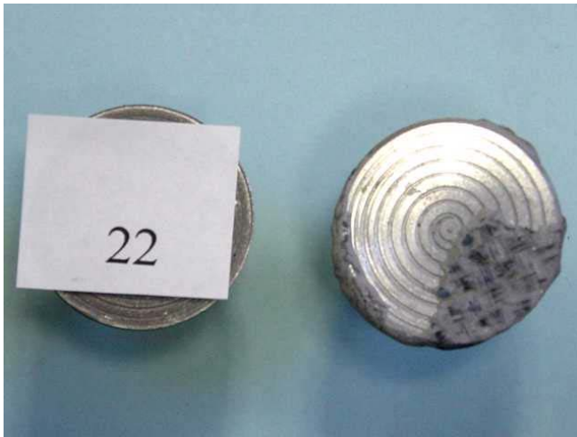
Figure 4.9: Example of separation at the plug bond.
