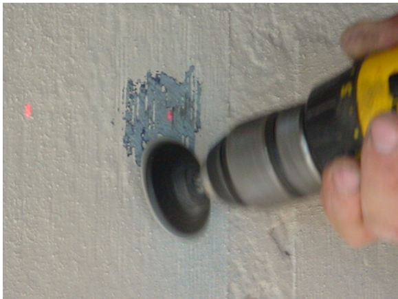
Figure 4.4: Pull-off test plugs are installed over the FRP sheets. First the surface is sanded, and then epoxy is used to bond the plug to the surface. Where location is critical, a positioning laser is used to precisely locate the position of the plugs.
