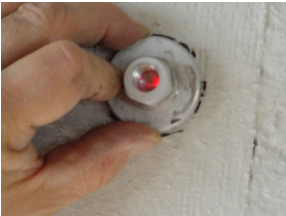
Figure 4.4: Pull-off test plugs are installed over the FRP sheets. First the surface is sanded, and then epoxy is used to bond the plug to the surface. Where location is critical, a positioning laser is used to precisely locate the position of the plugs.
