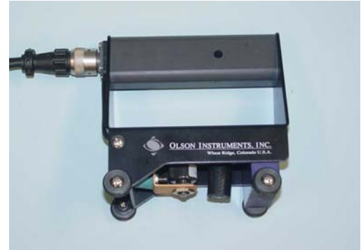
Figure 3.2: Impact echo tester modified with air coupled receiver.
