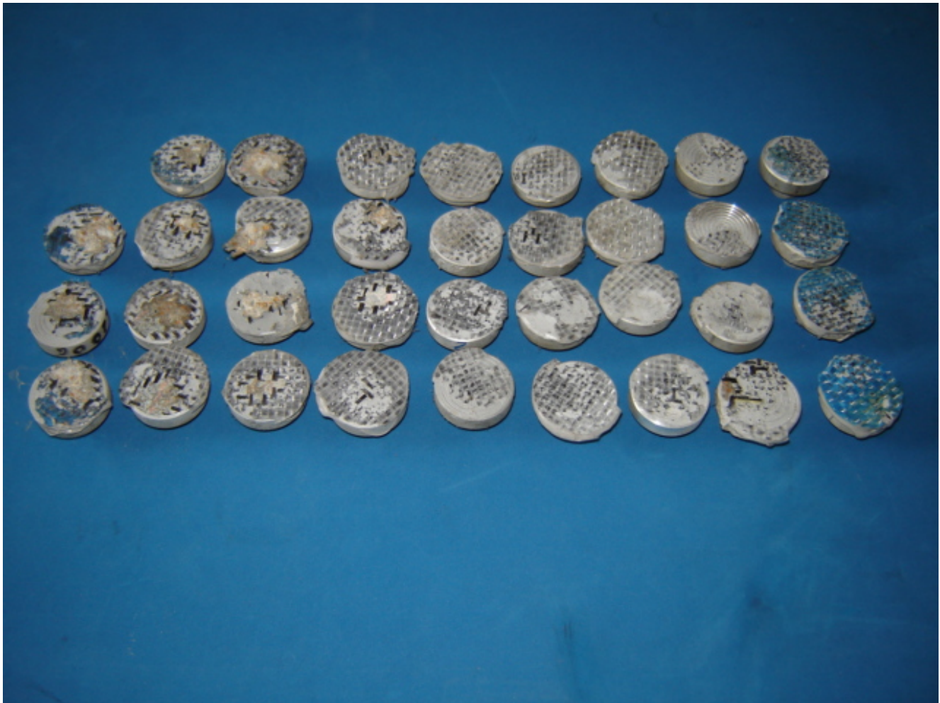
Figure 4.8: Failed pull-off plugs.
