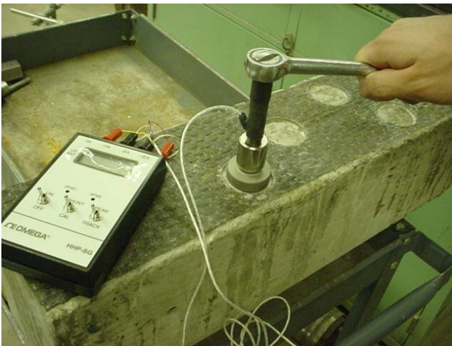
Figure 4.1: Pull-off tester used in a shear mode.
