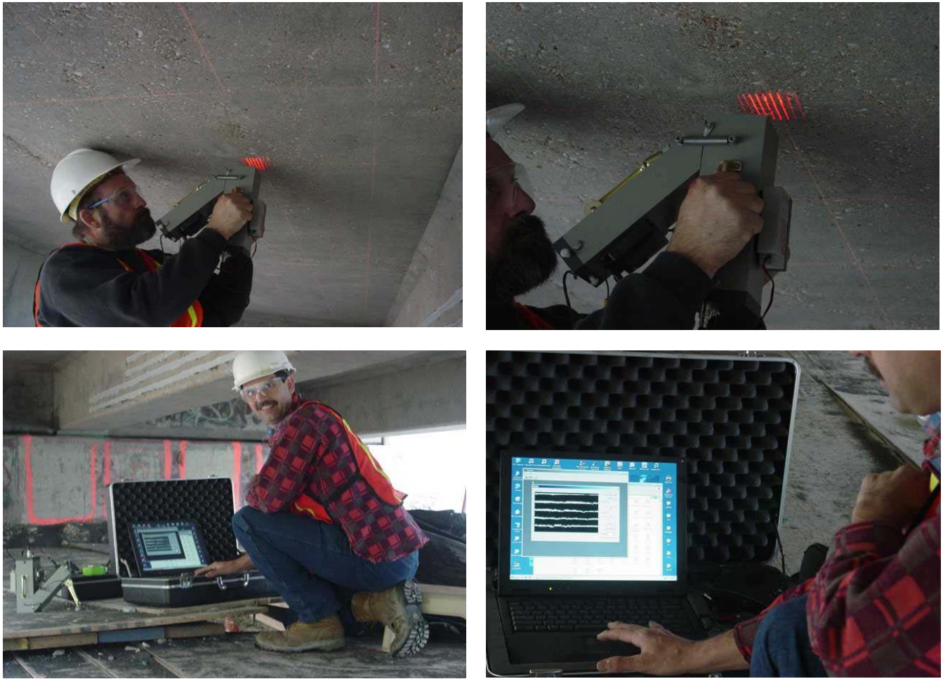
Figure 1.3: Using the laser profilometer under the gold bridge.
