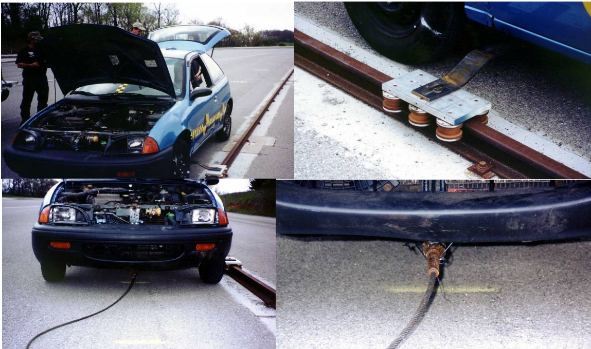
Figure 53. Bogey assembly and its attachment to vehicles.
