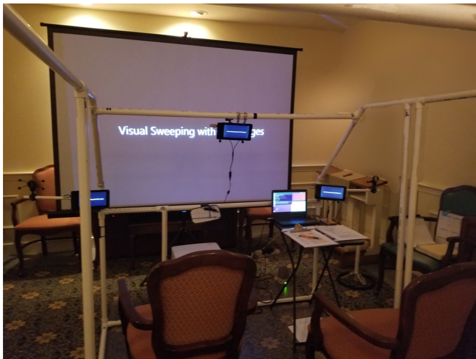
Figure 2. View of PVC car from the inside, with projection screen simulating forward roadway scene, and rearview and side mirror displays
