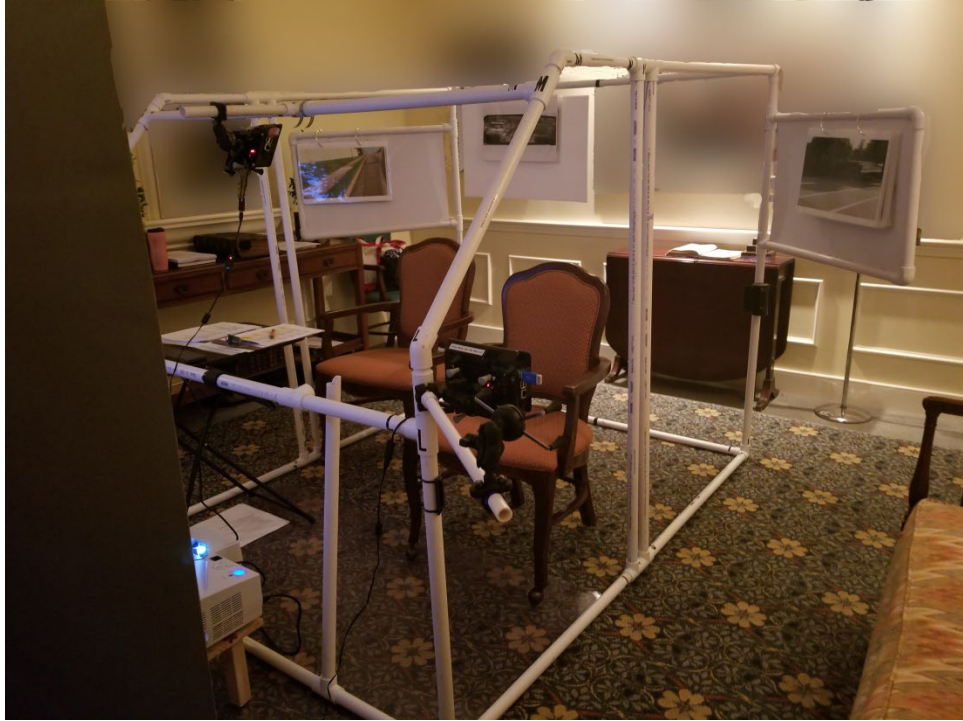
Figure 1. Front of PVC car viewed from the outside, showing driver and passenger positions and stimuli representing the roadway scene behind the vehicle
