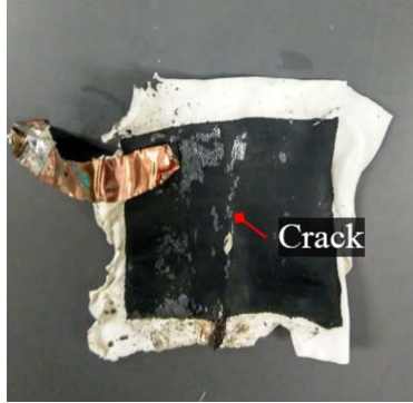
Figure 4.10: Damaged SEC a1 after Removal
