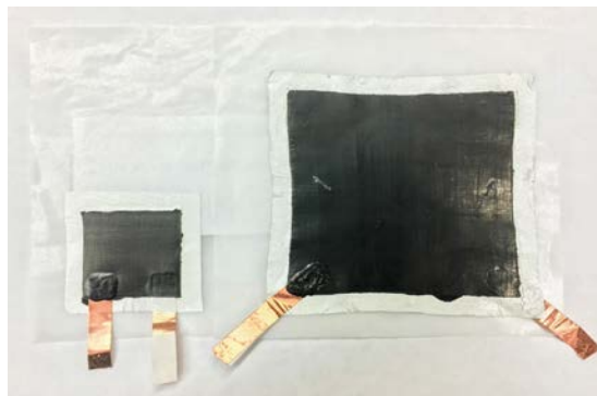
Figure 5.1: Two Sizes of SEC: 1.4 in. \times 1.4 in. (left); 3 in. \times 3 in. (right)
