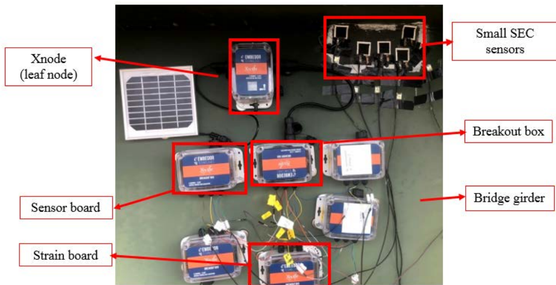
Figure 6.24: Sensor Layout of the Field Deployment on 07/16/2018 (Exterior Side of the Girder)
