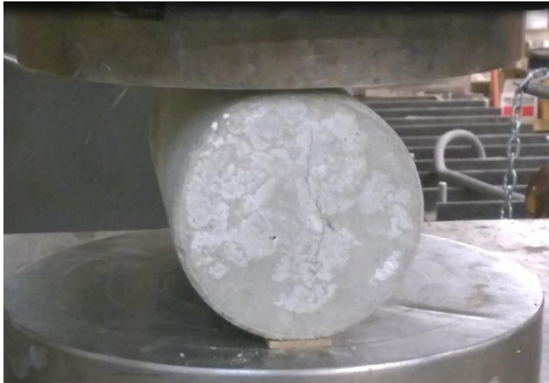
Figure 3.8 Splitting tensile test setup
