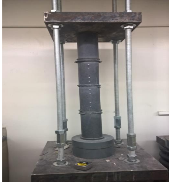
Figure 3.12 Creep testing frame
