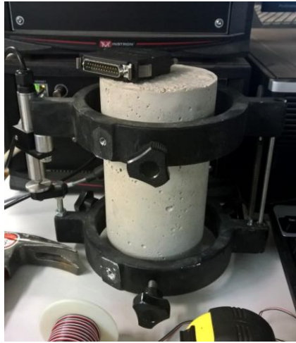
Figure 3.7 Extensometer cage for determination of modulus of elasticity
