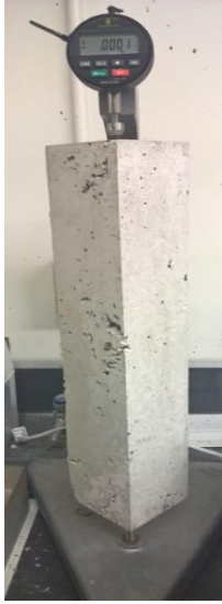
Figure 3.9 Length comparator for drying shrinkage measurement
