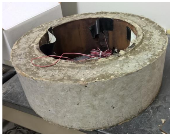
Figure 3.10 Restrained ring shrinkage test
