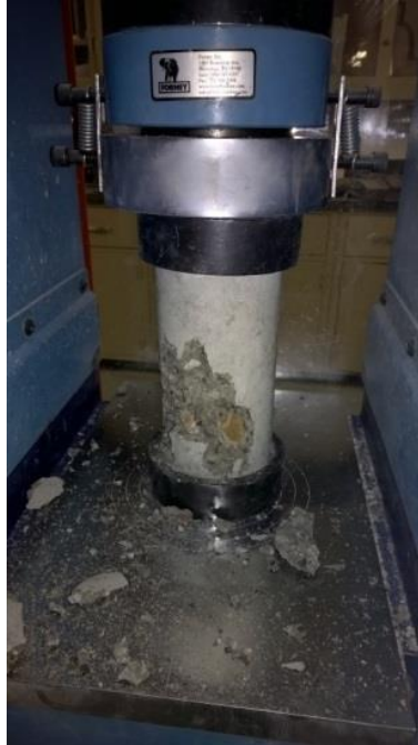
Figure 3.6 Compression testing setup
