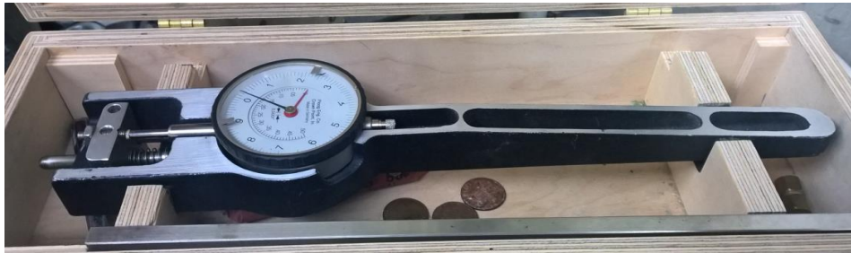
Figure 3.13 Creep strain measurement device
