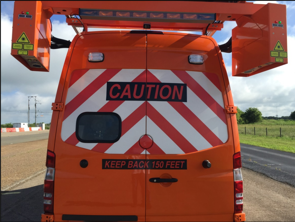
Figure 2. Scanning Lasers Mounted on Top Left and Top Right of ARAN Unit.
