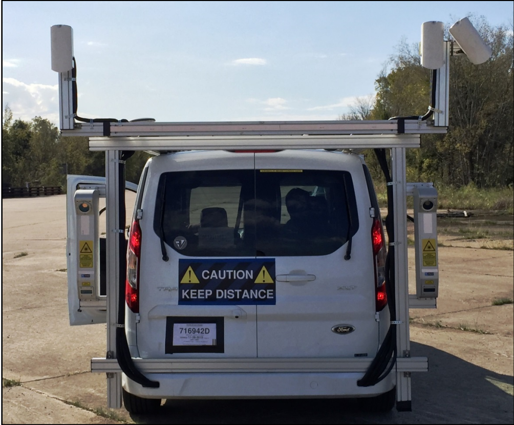
Figure 1. Scanning Lasers Mounted on Each Side of D-Vision Test Vehicle.
