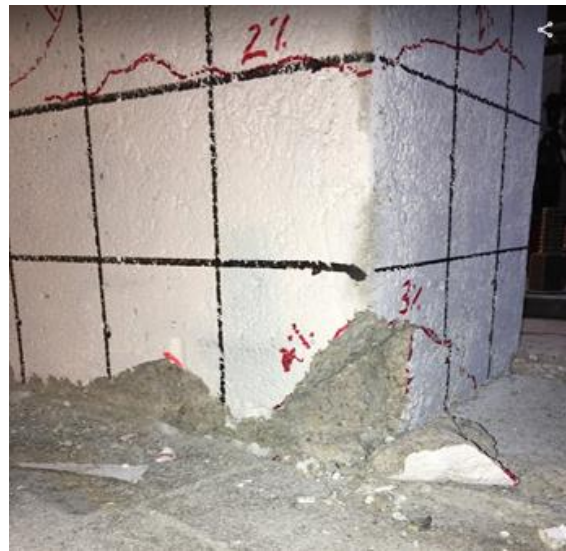
Figure 3.10 Spalling at 4% drift of as-built wall pier
