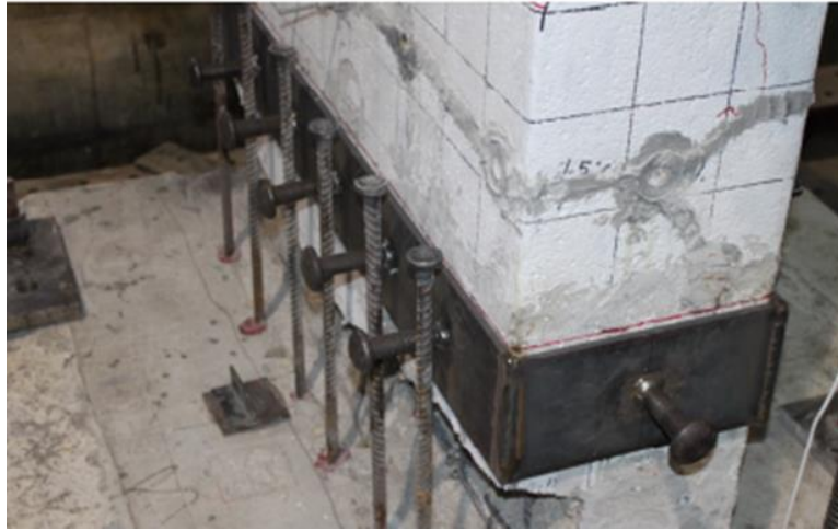
Figure 8.4 Steel collar with welded studs for specimen MCRP
