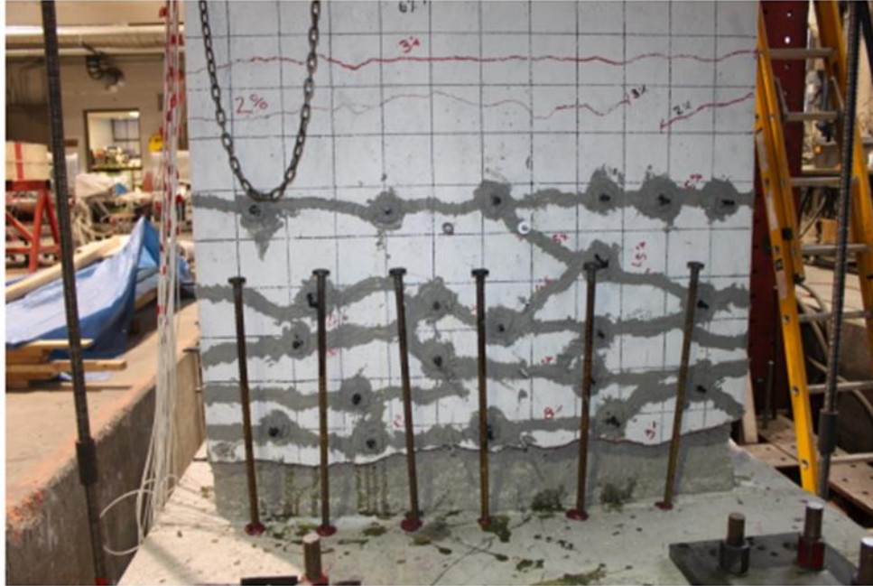
Figure 8.3 Installed headed steel bars for repaired specimen MCRP
