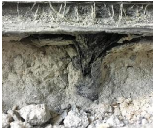
Figure 5.11 Partial anchor fracture for Specimen R1
