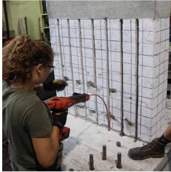
Figure 7.2 Mild steel NSM bar placement for specimen ABRP
