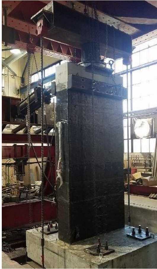
Figure 6.3 Specimen R2 with the final retrofit application
