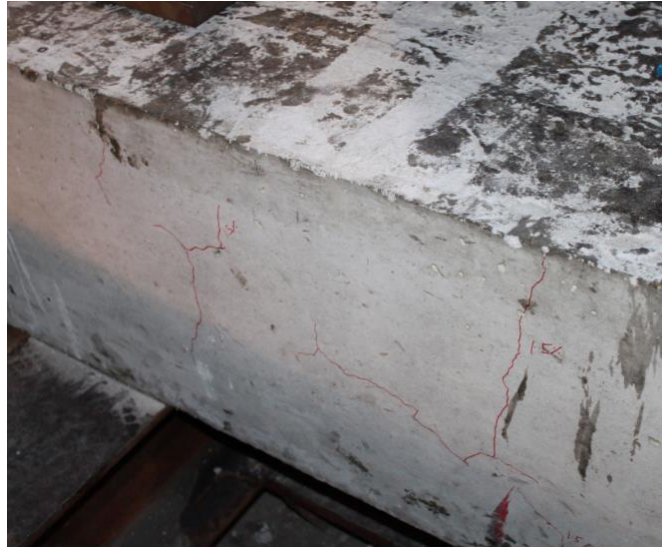
Figure 7.11 Footing cracks at 1.5% drift ratio for specimen ABRP
