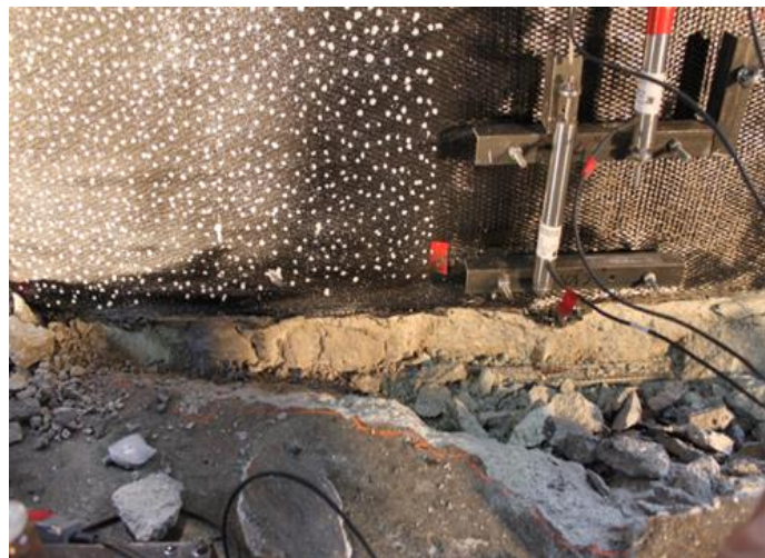
Figure 5.13 Footing damage at the end of the test for specimen R1
