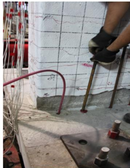
Figure 8.6 Headed steel bar installation process: (left) drilling holes; (right) headed bar placement for specimen MCRP
