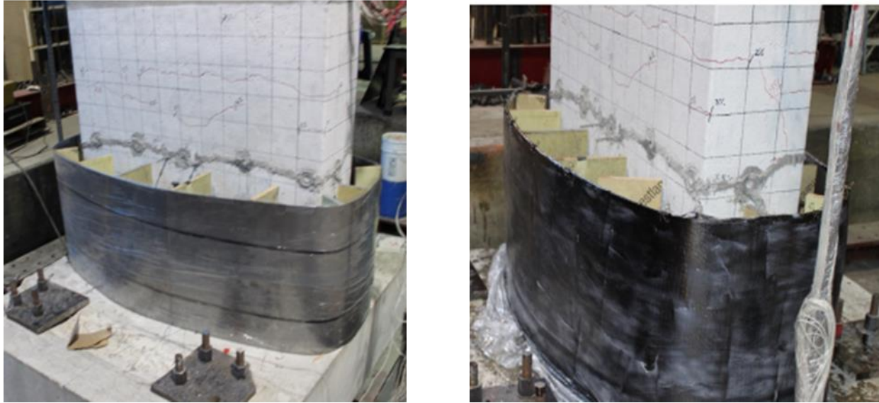
Figure 8.7 CFRP donut formation: (left) shell formation with precut aluminum foil; (right) CFRP wrapped around the aluminum form
