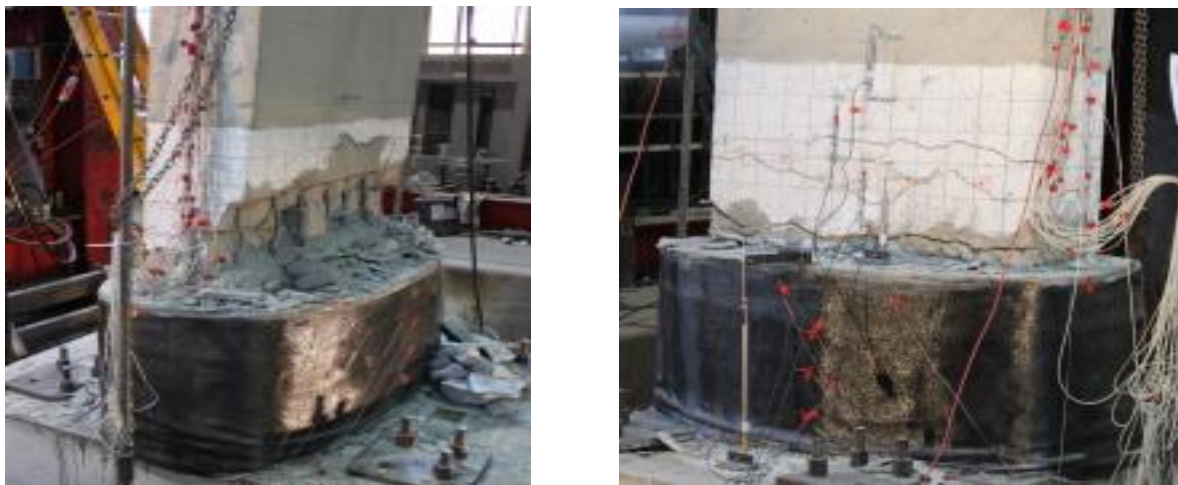
Figure 8.14 Experimental observation of specimen MCRP at a 5% drift ratio: (a) east side (b) west side
