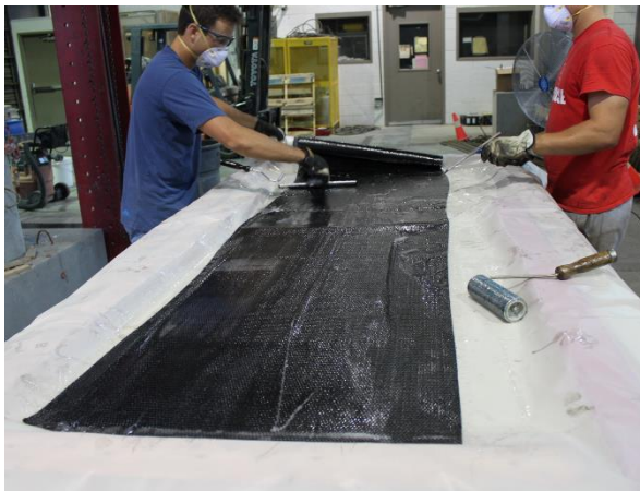
Figure 7.4 Repair application process for specimen ABRP: (a) fiber saturation, (b) hoop direction CFRP wrap application, (c) horizontal CFRP anchors, (d) final wall repair
