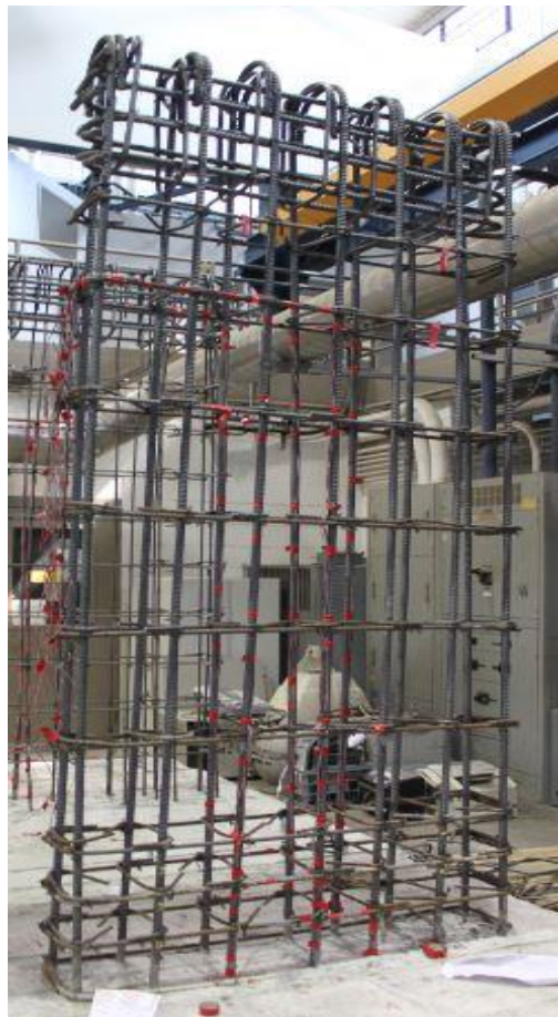
Figure 2.9 Code compliant wall pier reinforcement
