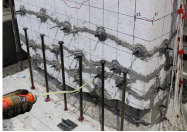
Figure 8.5 Epoxy injection of cracks for specimen MCRP
