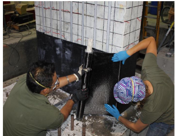
Figure 7.4 Repair application process for specimen ABRP: (a) fiber saturation, (b) hoop direction CFRP wrap application, (c) horizontal CFRP anchors, (d) final wall repair
