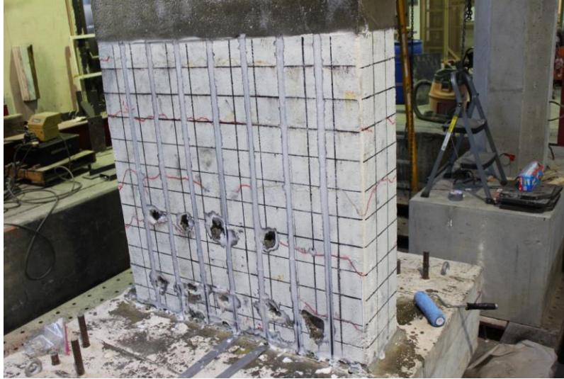
Figure 7.3 Epoxy coverage of steel NSM bars of specimen ABRP
