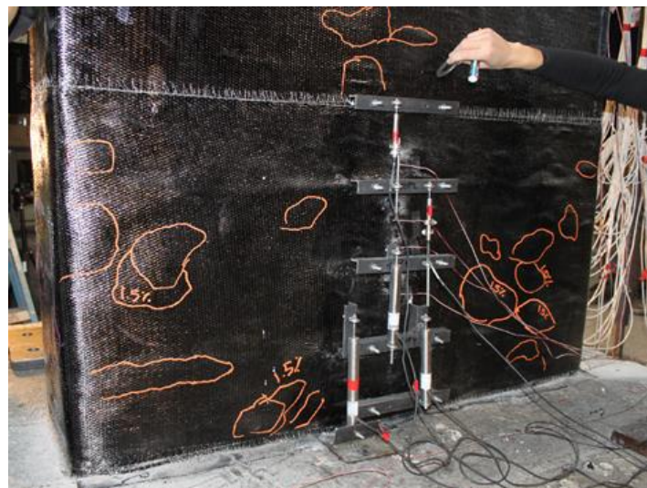
Figure 5.10 CFRP jacket debonding at 1.5% drift ratio for specimen R1
