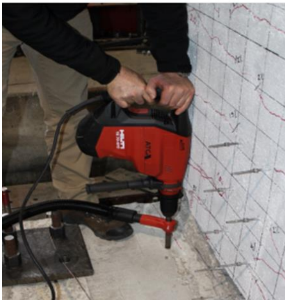
Figure 8.6 Headed steel bar installation process: (left) drilling holes; (right) headed bar placement for specimen MCRP
