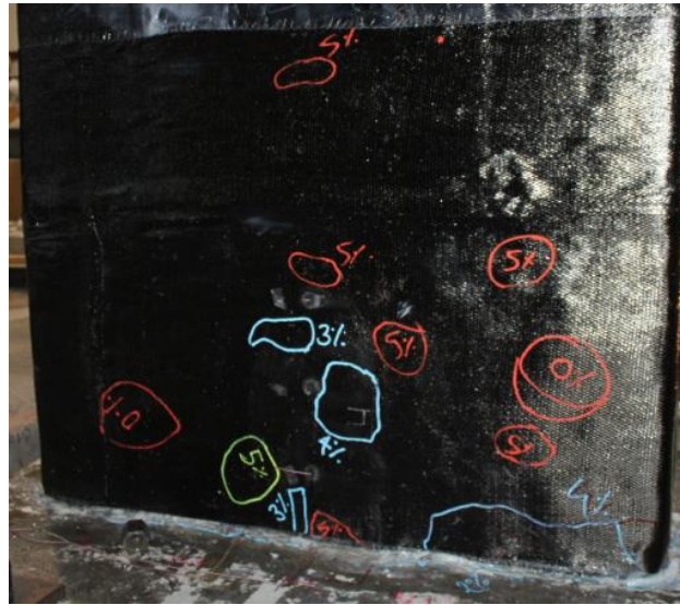
Figure 7.12 West face CFRP wrap debonding at 4% drift ratio for specimen ABRP
