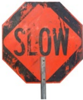
Damaged slow paddle sign (MoDOT)
