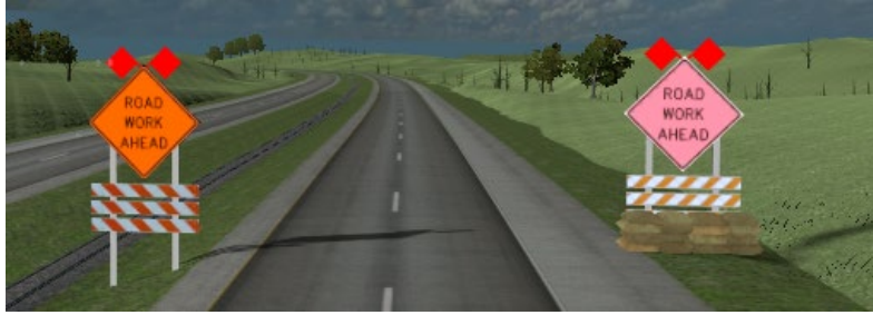
Right side sign pink color or faded and large mound of sandbags
