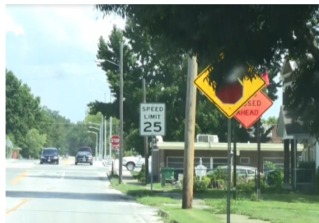
Signs obstructed by tree and other sign (MoDOT)
