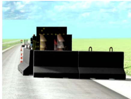
TMA hidden by concrete barriers (virtual reality)
