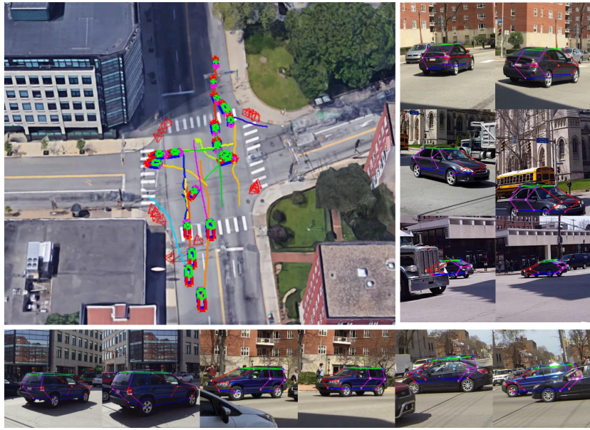
Figure 2: Reconstruction of vehicles crossing a busy intersection, making turns, going straight and changing lanes. A subset of vehicle skeletons (3D detector locations) and their 3D trajectories are augmented within the Google Earth view of the intersection. The reconstructions are reprojected into multiple views of two cars (a sedan and an SUV) demonstrating good performance under partial occlusions.
