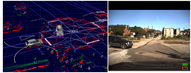
Fig. 17: The autonomous vehicle stops at a four-way-stop intersection, and waits for its turn to move
