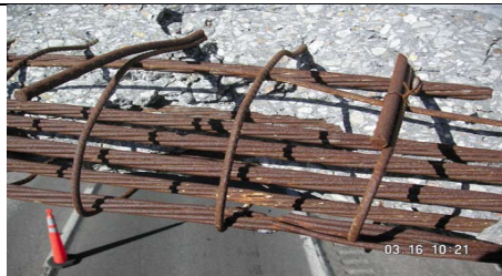
Figure 7: Severe I damage, one severed strand, NDOT Wood River Interchange Bridge Girder (A)
