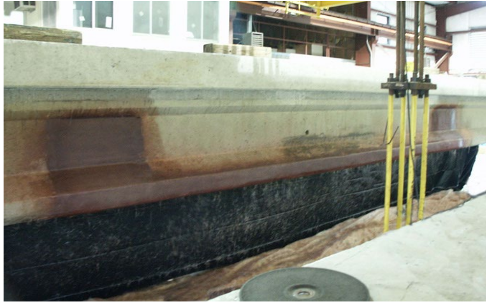
Figure 37: Repaired specimen, courtesy of Boyd et al, 2006
