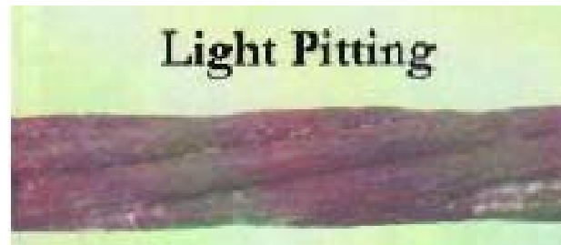
Figure 5: Extensive damage, exposed strands having corrosion with light pitting, Naito et al., 2006
