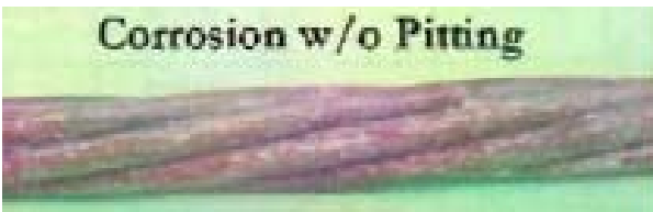
C: Corrosion without pitting
