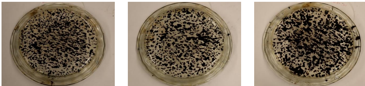
Figure 88. Pie Plates (With Loose Mixture) of GRN3 Mixtures with PG 67-22 Binder at (a) JMF OBC-0.5% (6.0%), (b) JMF OBC (6.5%), (c) JMF OBC+0.5% (7.0%)
