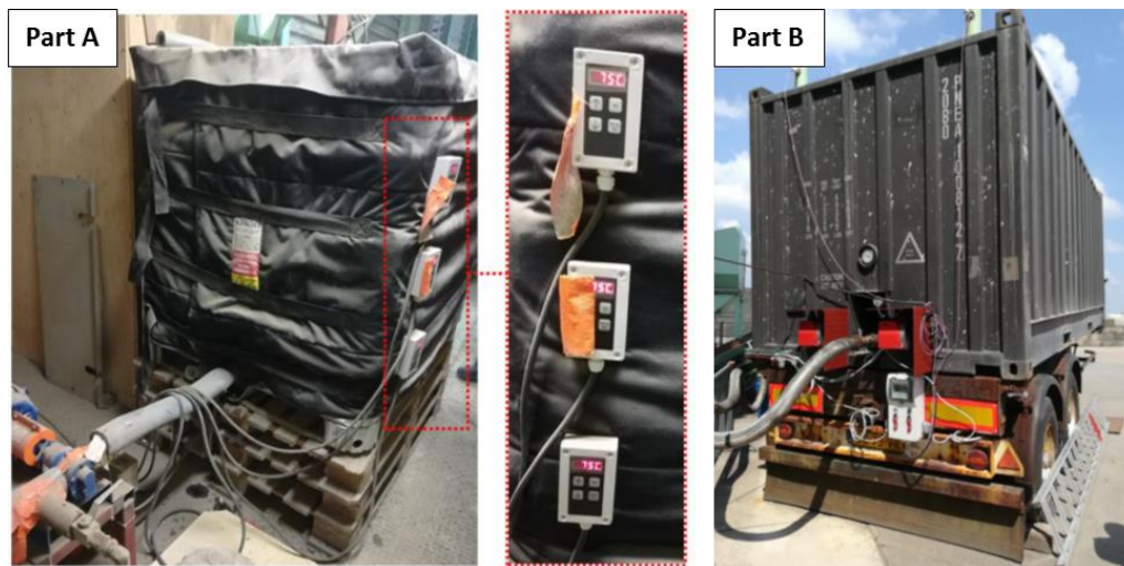
Figure 27. Introduction of Epoxy Asphalt Components at a Batch Plant in the Netherlands (Zegard et al., 2019)
