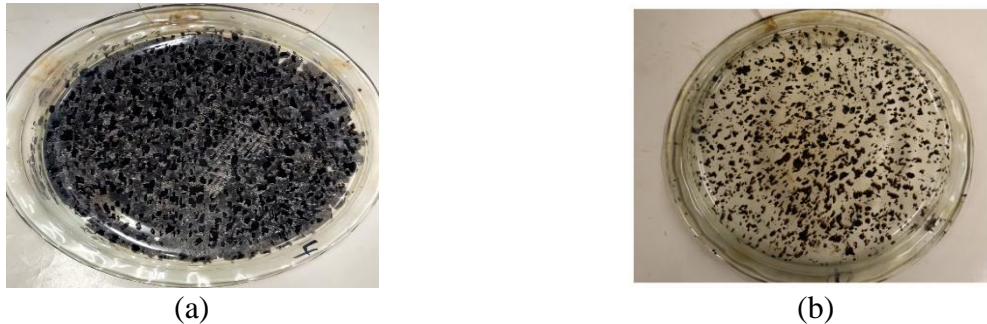
Figure 90. Pie Plates of GRN3 Mixture with J30Z EMA Binder at JMF OBC (6.5%): (a) With Loose Mixture, (b) Without Loose Mixture
