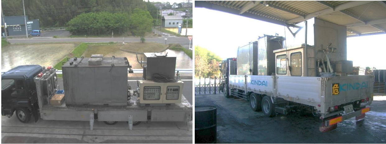
Figure 29. Epoxy Materials Distributing Truck in Japan
