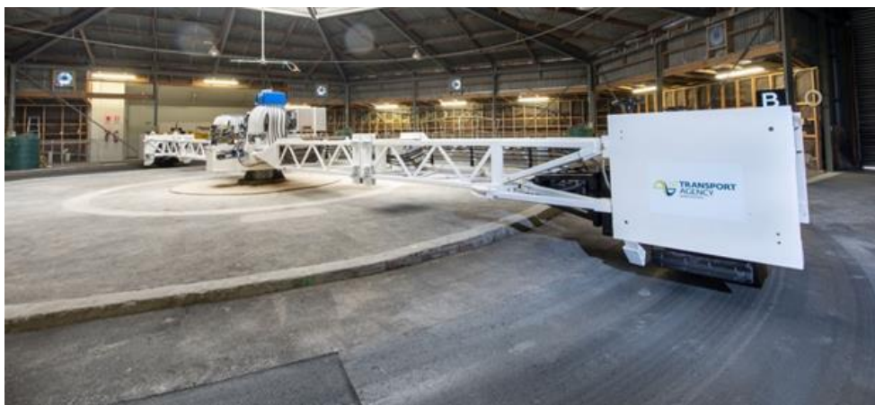
Figure 17. EMA OGFC Test Section at CAPTIF (Herrington et al., 2007)
