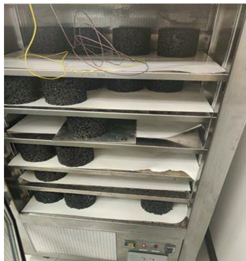
Figure 49. Aging of Compacted OGFC Mixture Specimens in the Environmental Chamber
