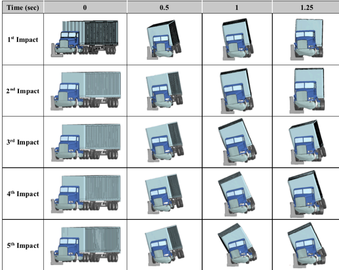
Figure 4. Frame comparison of impact simulations for Manitoba concrete bridge rail – front view
