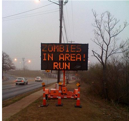
Figure 2.3 A compromised DMS from an online guide on exploiting DMSs [77]
