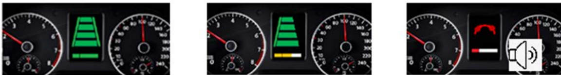
Figure 4. Automation displays full confidence in solid icons (left); automation displays mid-confidence in solid icons (center); automation displays low confidence with solid icons and auditory warning (TOR) (right)
