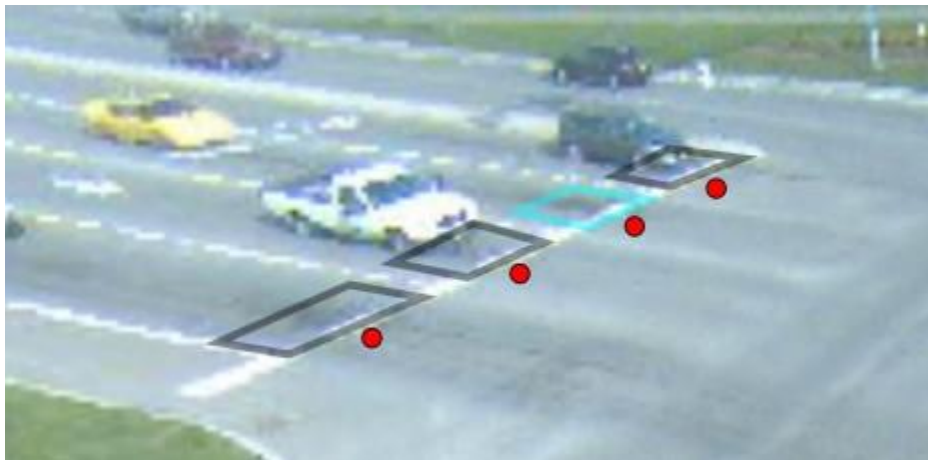
Figure 16. GS Software View of the Intersection Approach Showing Vehicles and Detection States
