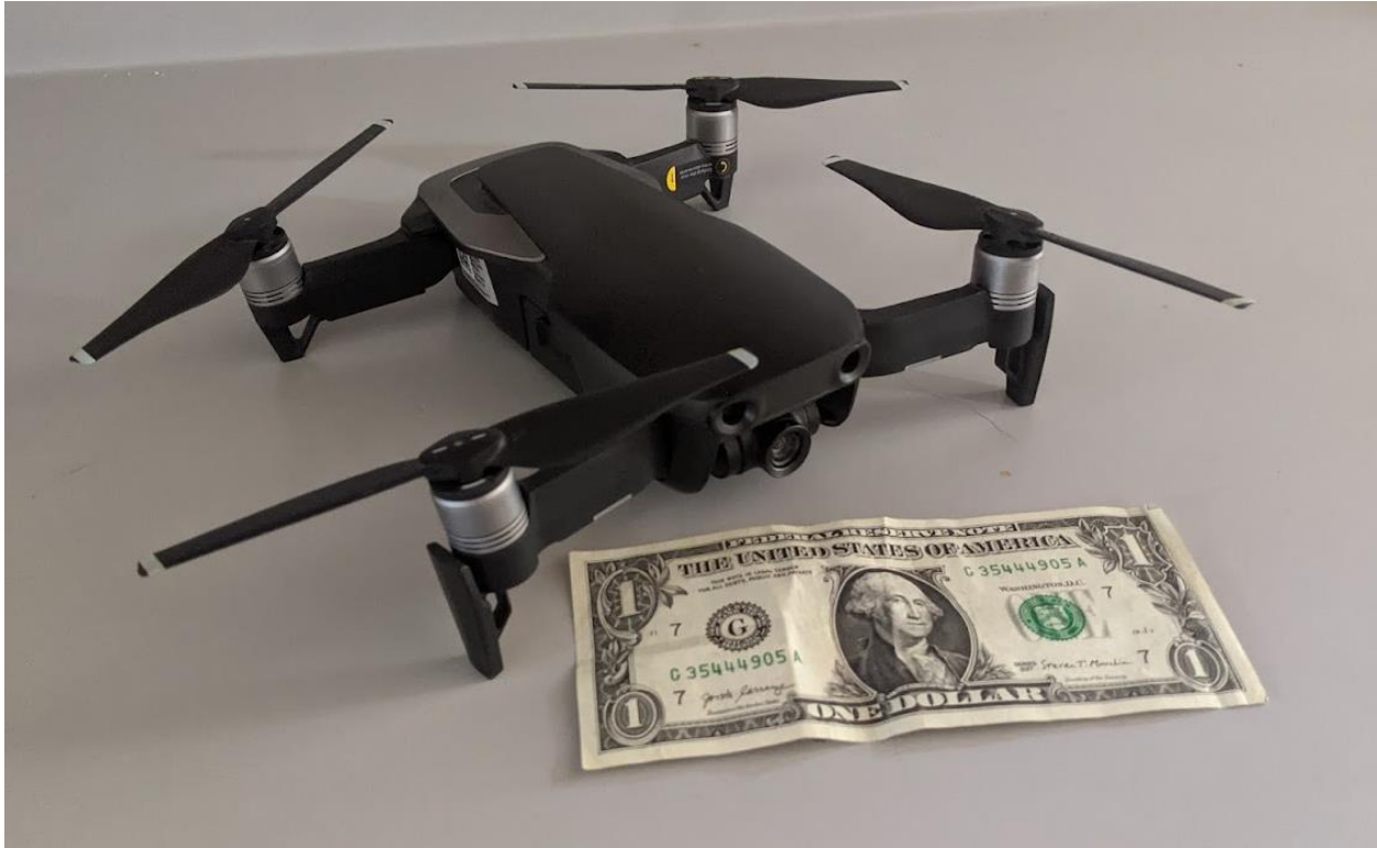
Figure 9. DJI Mavic Air® UAV of the Type Used for Aerial Video Collection at the Intersections
