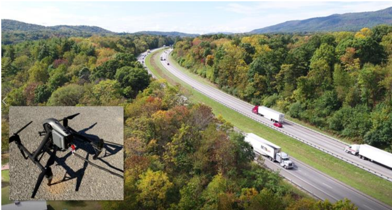
Figure 4. Video View Collected by the Tethered DJI Inspire 2 UAV (Inset) of I-81 Near Salem, VA
