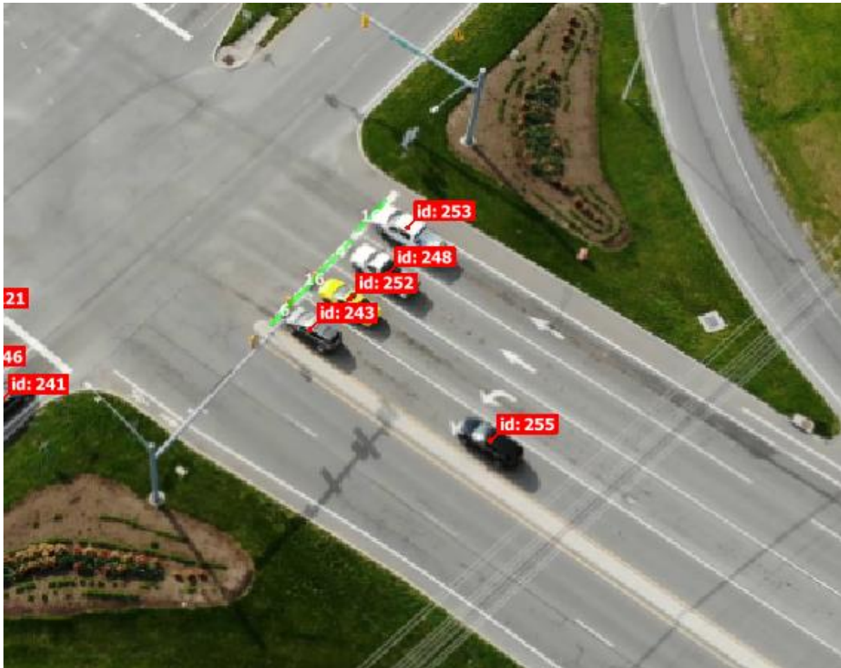
Figure 14. Screen Capture from the DFS Viewer of the SR 114 Eastbound Approach Looking Southeast and Showing the Four Virtual Gates and Respective Vehicle Identification Numbers in Red and Vehicle Count Numbers Embedded Within the Green Gates
