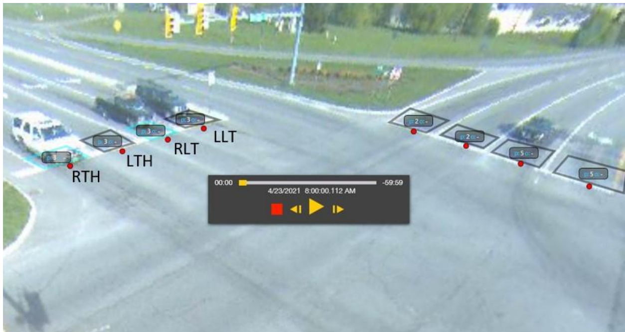
Figure 13. GS Camera View of SR 114 Eastbound and North Franklin Southbound Approaches Looking Northwest and Showing Vehicle Detection Zones, Viewing Tool Play Controller with Time and Lane Labels
