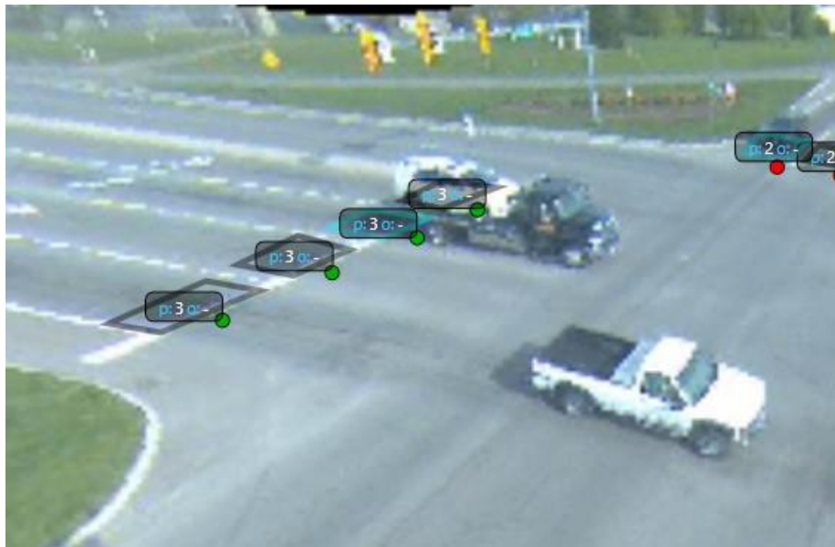
Figure 18. GS Software View of the Intersection Approach Showing Vehicles and Detection and Count States
