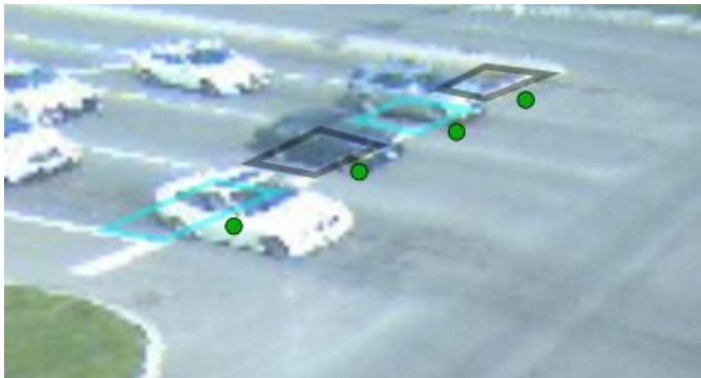
Figure 19. GS Software View of the Intersection Approach Showing Vehicles and Detection States
