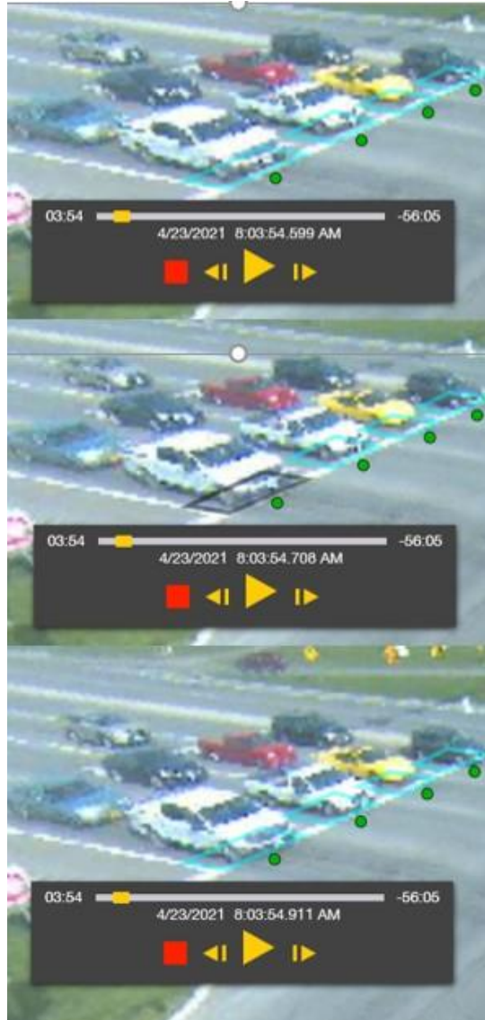
Figure 15. GS Software View of the Intersection Approach Showing Vehicles and Detection States
