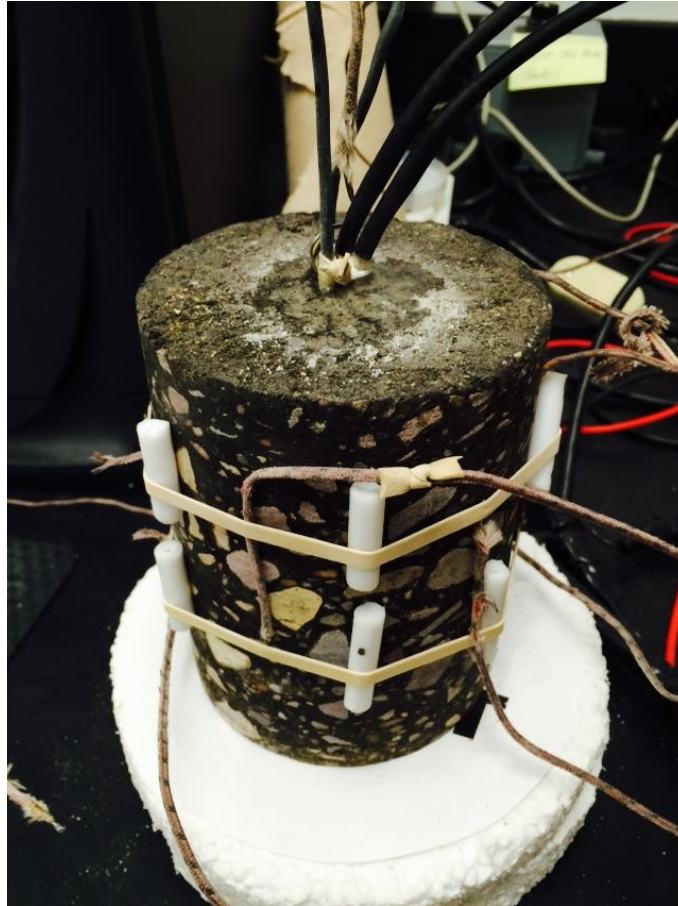
Figure 147. Thermal conductivity test specimen before upper insulation
