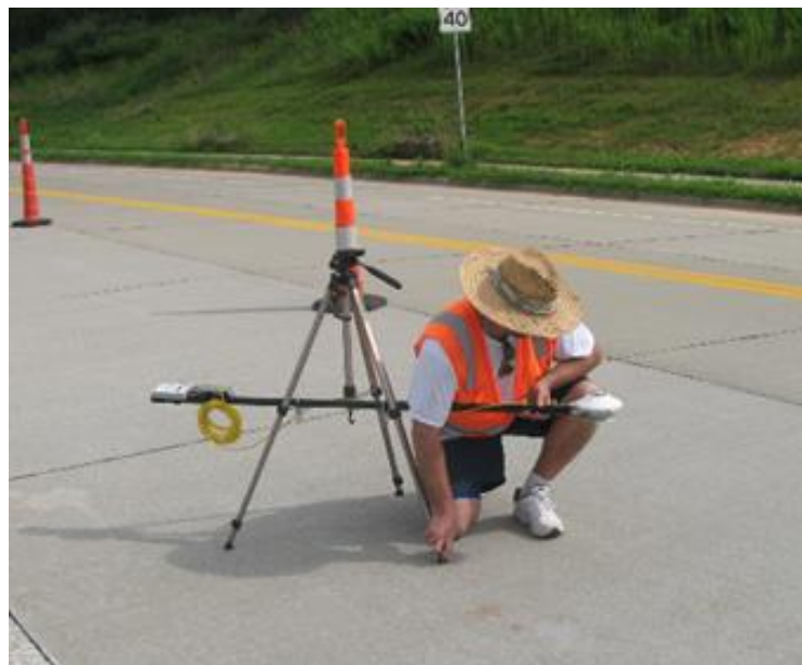
Figure 34. Albedometer mounting during city field testing
