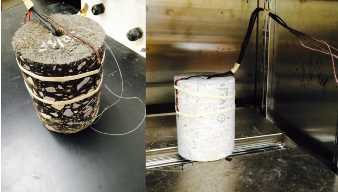
Figure 154. Prepared specimens for heat capacity test
