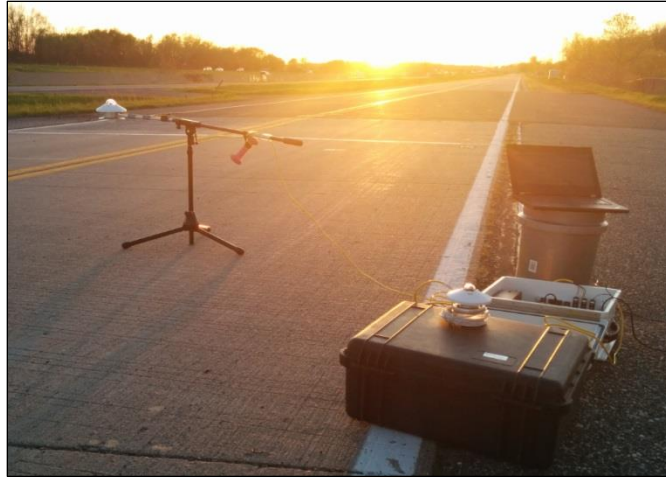
Figure 1. Pavement albedo assessment - MnROAD test track site
