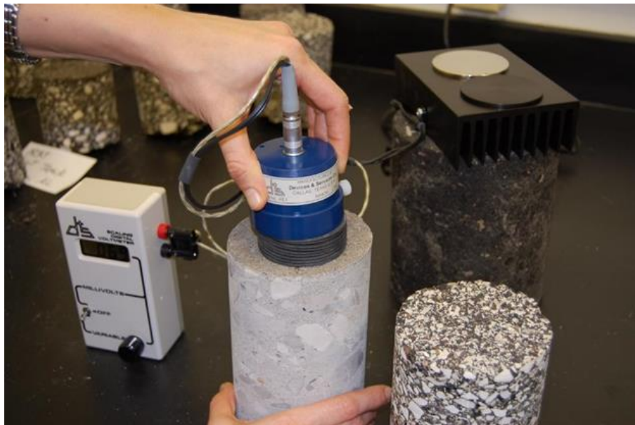
Figure 45. Emissivity laboratory testing setup
