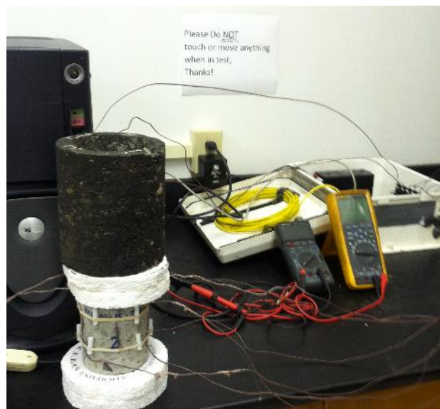
Figure 42. Thermal conductivity laboratory testing setup and data collection
