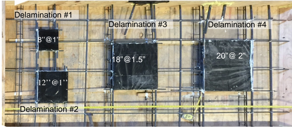
Figure 4-1 Concrete specimen with four artificial delaminations
