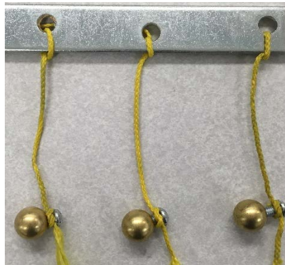
Figure 4-10 Three parallel metal balls as excitation source
