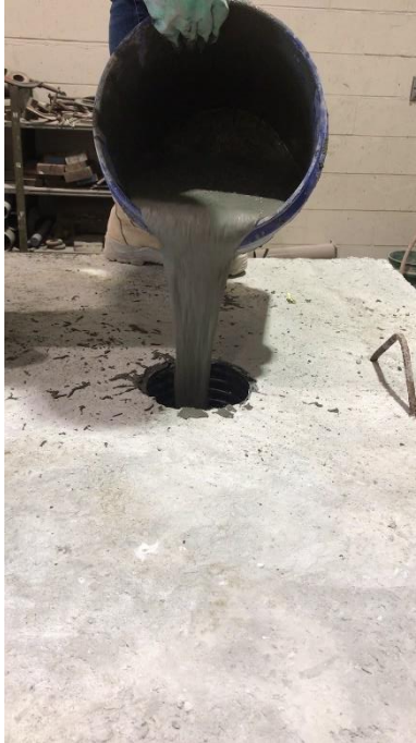
Figure 4.034: UHPC Casting for UHPC#2 Specimen.
