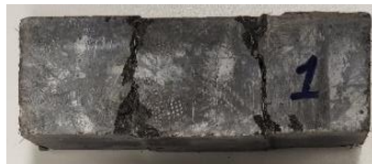
Figure 4.02: Double Shear Failure Mode of Direct Shear Test Specimen.
