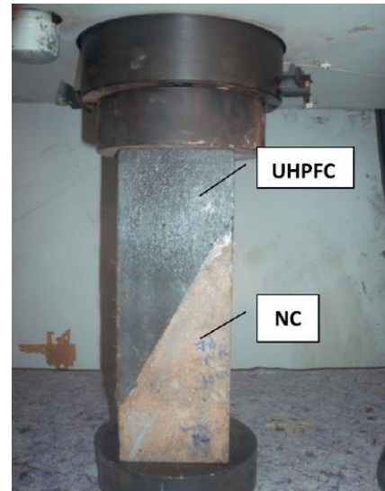
Figure 2.16: (a) Mix Proportions of UHPFC and CC, (b) Surface Textures, and (c) Test Configuration (Tayeh et al. 2012)
