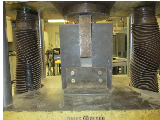
Figure 4.01: Direct Shear Test Setup.
