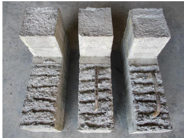
Figure 4.024: Interface Surface Roughening and Different Reinforcement across Interface; No Reinforcement (Left), 2leg No. 3 Stirrup (Middle), and 2leg No. 4 Stirrup (Right).
