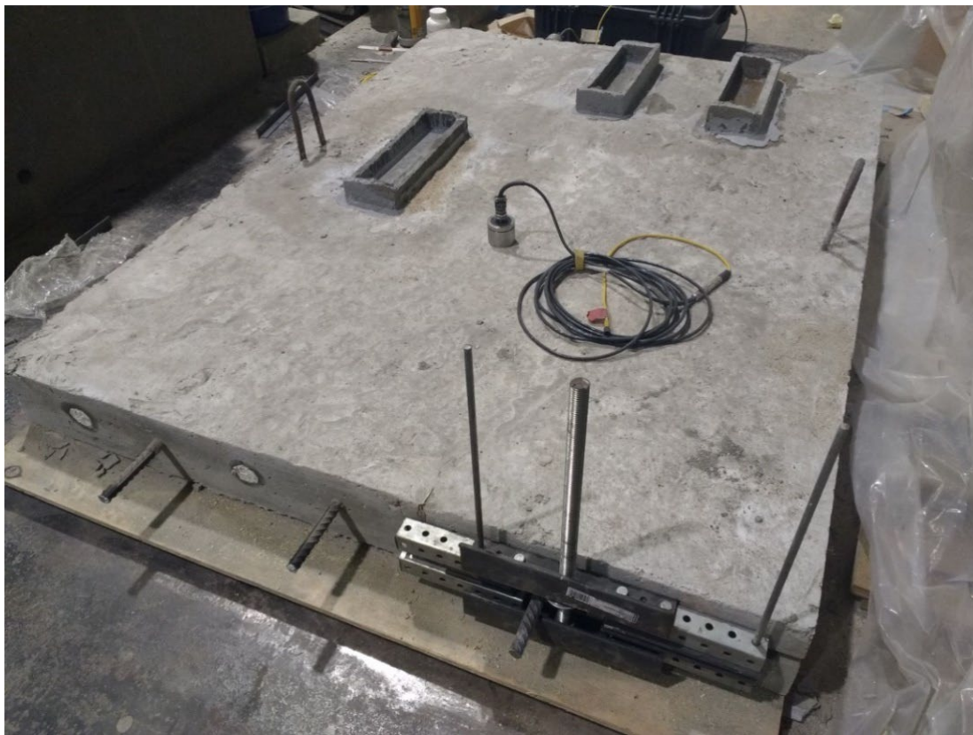
Figure 3- Specimen Set 1B (Corrosion-delamination Specimens)
