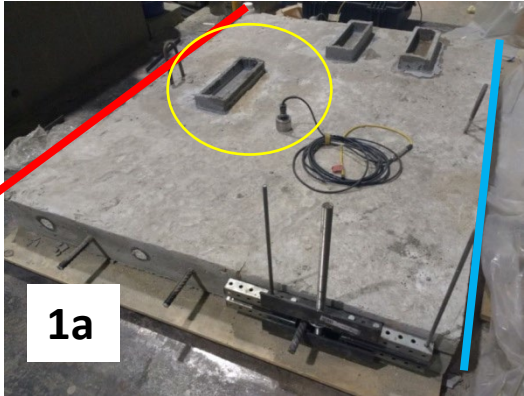
Figure 12- Red line denotes the sensor array for data displayed in Figure 11, and blue line denotes the sensor array for data displayed in Figure 14.
