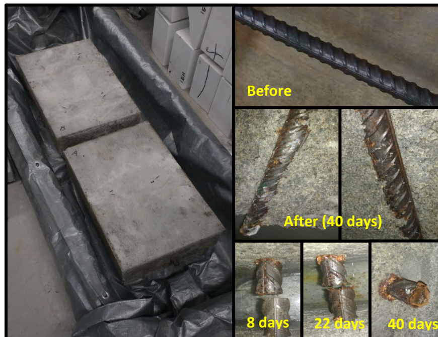
Figure 2 – Specimen Set 1A: Corrosion Specimens (left) and Corrosion product build-up over time (right)
