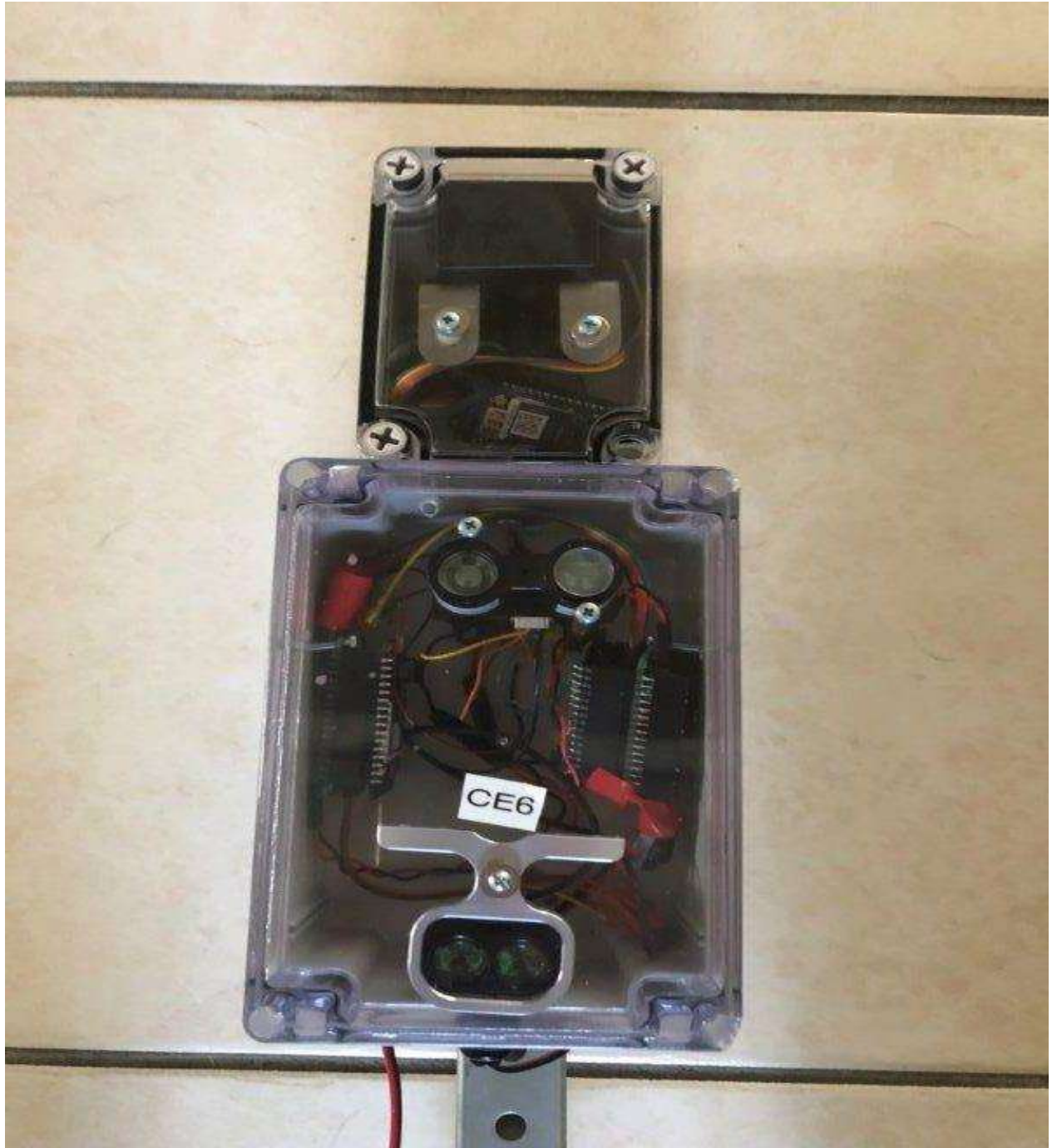
Figure 102: Capture Unit with Three Different Sensors
