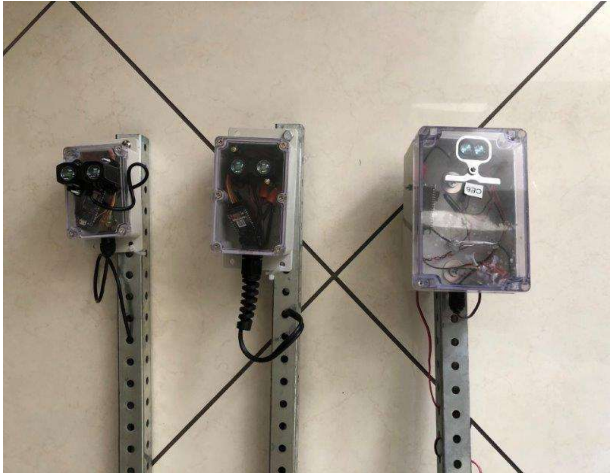
Figure 101: Three Complete Capture Units
