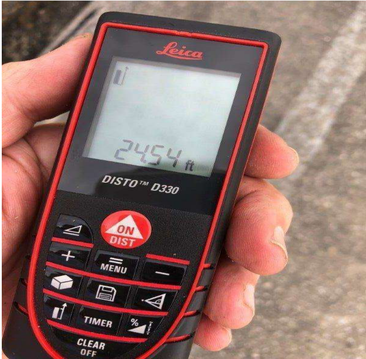
Figure 114: Distance from Sensor to Highway below
