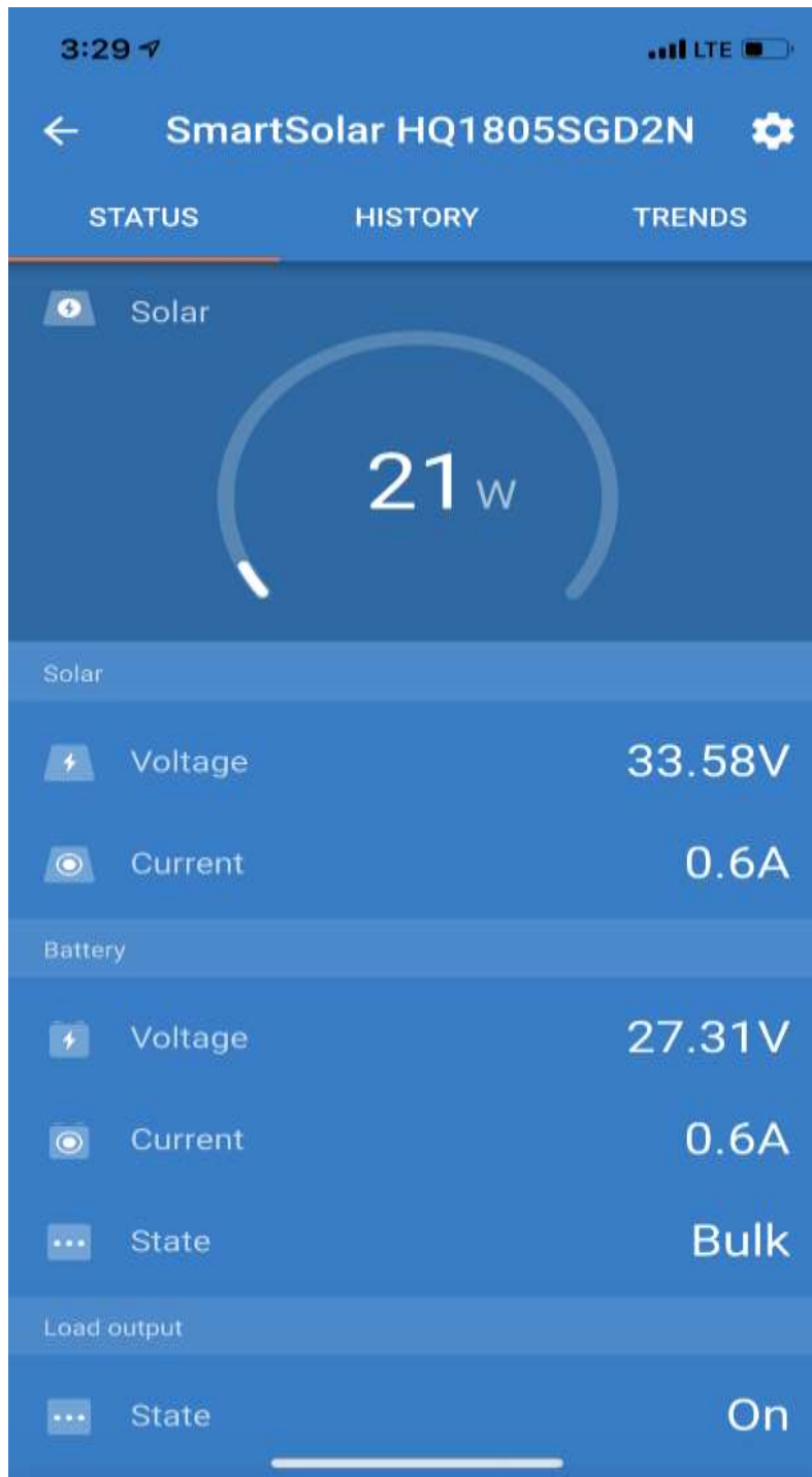
Figure 110: Solar Controller Display via Bluetooth
