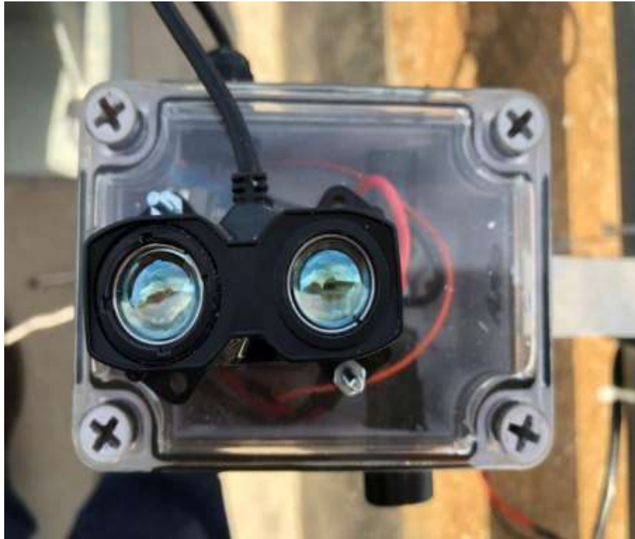
Figure 72: New Laser Sensor (High Frequency)
