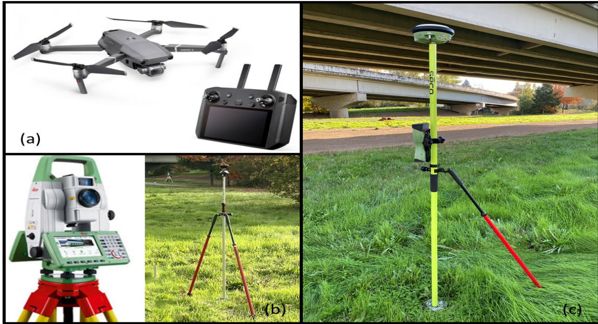
Figure 4.2. Equipment used in this study: (a) DJI Mavic 2 pro and the smart controller; (b) Leica Nova MS50 MultiStation, prism, and adjustable height pole and bipod; (c) Leica GS14 GNSS receiver, Leica CS15 data collector, fixed height pole and bipod.
