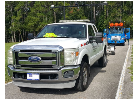
The ATMA leader vehicle and the driverless follower vehicle are connected by several types of communications.
