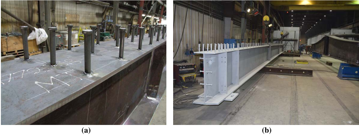
Figure 18. Carbon Steel Shear Studs: (a) top flange of beam; (b) top flange and web after mill scale removal
