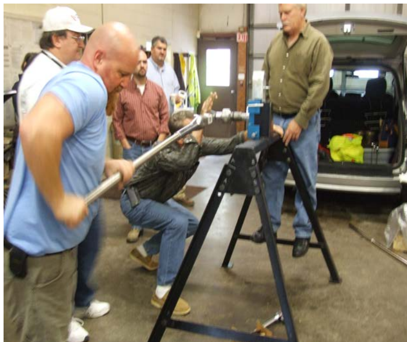
Figure 24. Acceptance Testing of ASTM A193 Grade B8 Class 2 Bolts
