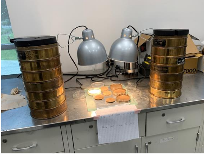
Figure 4. Setup of the cyclic wetting and drying tests.
