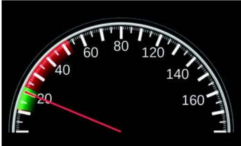
Figure 2: One of the GLOSA interfaces suggested for motor vehicles. The green band places the driver in the green wave.
