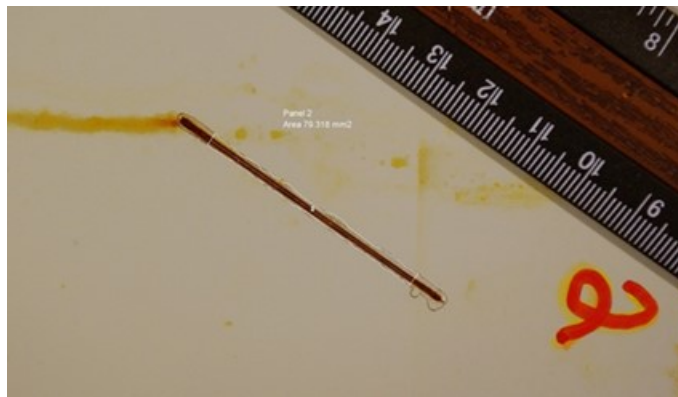
Figure 15. Sketching Rust Creepage Outline on Image
