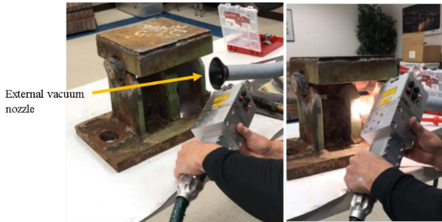
Figure 8. Images of Right-Angle CleanCUBE Head Geometry Processing in Tight Geometric Areas
