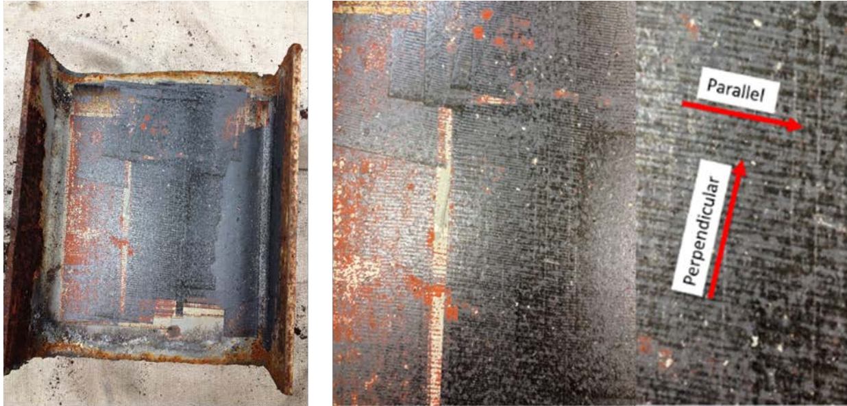
Figure 17. Photographs of Laser-Cleaned Area: (left) laser “tracks” left behind on surface after laser ablation; (right) higher magnification of region between tracks of random surface pattern of darker- and lighter-colored regions. Surface roughness was characterized parallel and perpendicular to the laser tracks.
