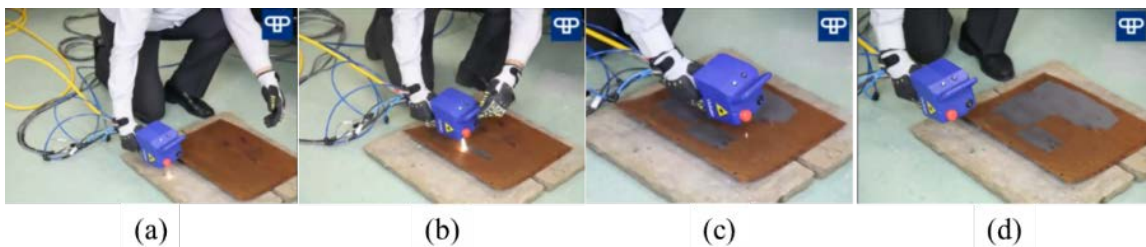
Figure 52. Demonstration of Powerlase 1.6 kW Vulcan Laser Head in Operation. Note compact and lightweight design.
