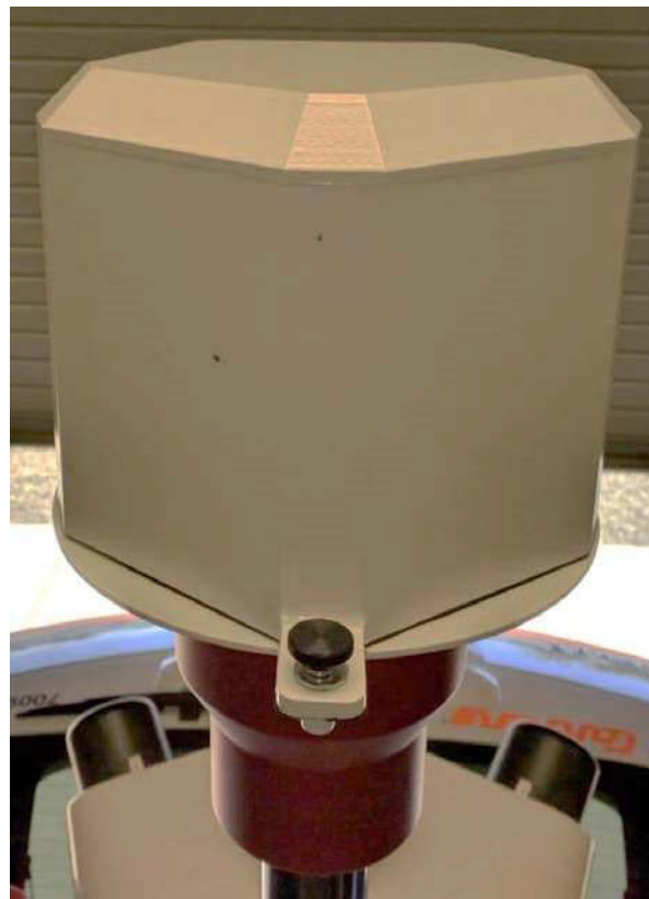
Figure 7.6: Custom 3D-printed Ladybug camera cap 3D-printed by DOE staff
