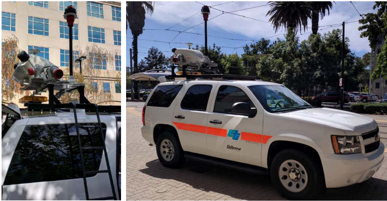
Figure 7.3: Riegl VMX-1HA sensor pod mounted on a custom roof rack with a Rhino-brand folding ladder on the side of the vehicle
