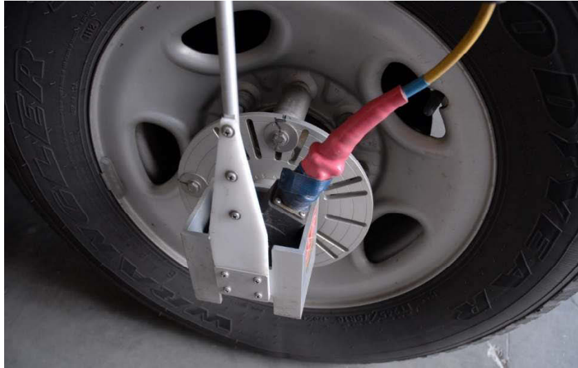
Figure 2.2: MTLS system DMI mounted on the driver-side rear wheel
