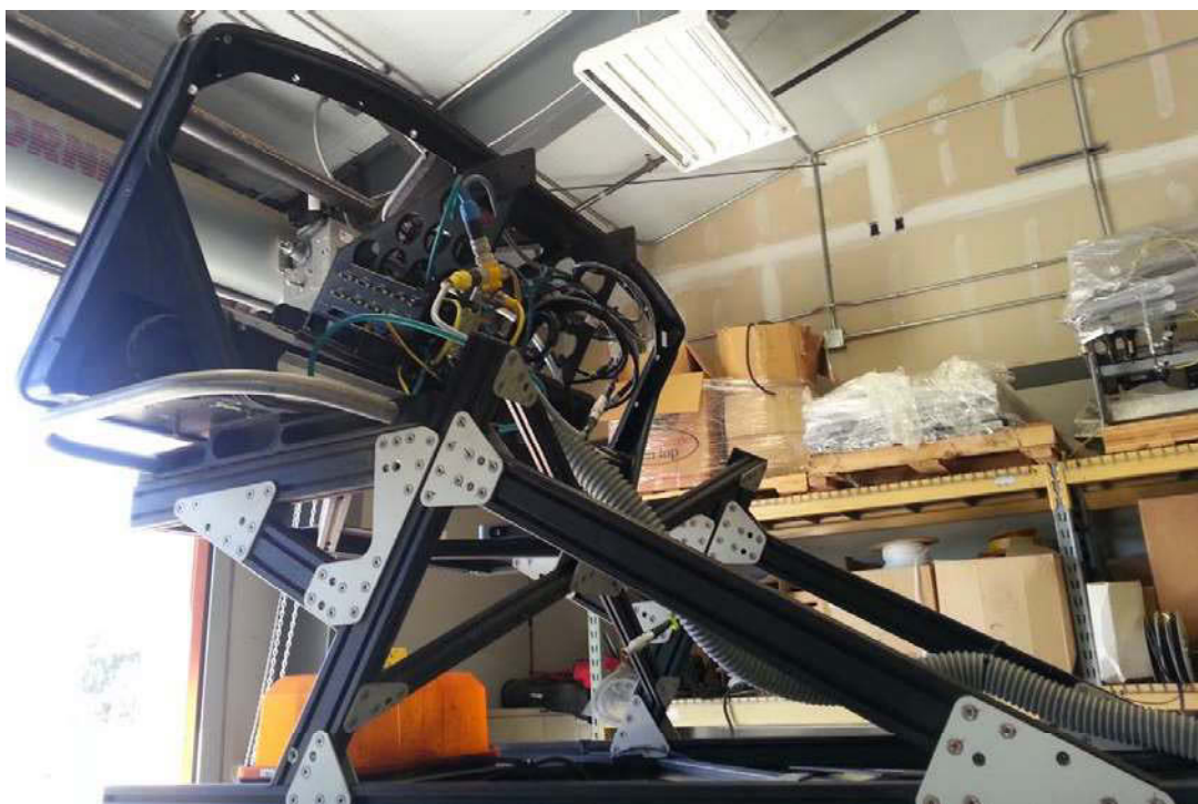
Figure 2.4: Sensor pod frame with the camera pods and laser scanners removed
