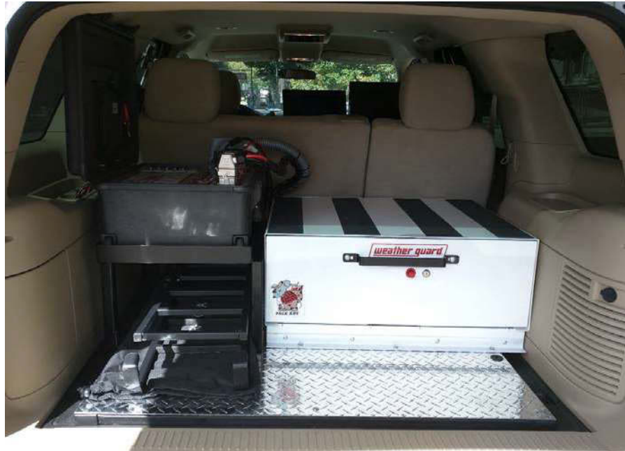
Figure 7.5: Riegl VMX-1HA control unit housed in a black Pelican case next to a white Weather Guard toolbox mounted at the rear of the Chevrolet Tahoe
