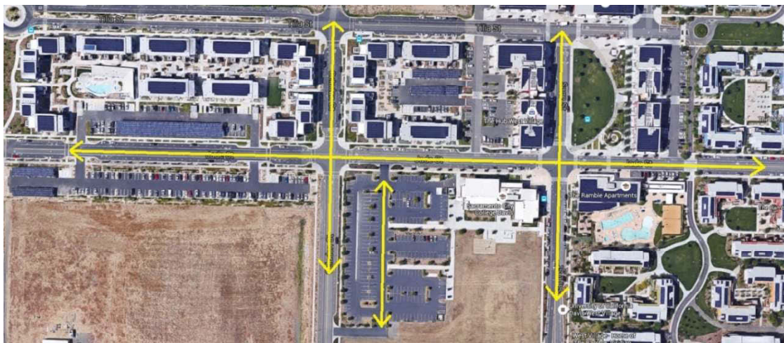
Figure 2.9: Google Map aerial image of UC Davis West Village used for MTLS calibration. Yellow lines are the recommended vehicle drive paths.
