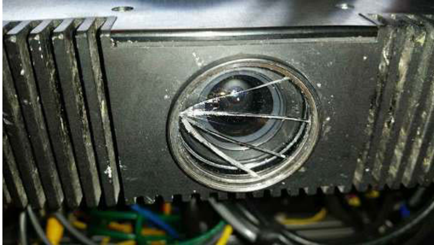
Figure 2.6: Broken front-center camera filter from shipping
