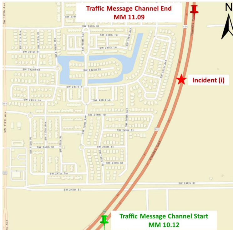
Figure 4-3: An Example of Assigning Incidents to Traffic Message Channels
