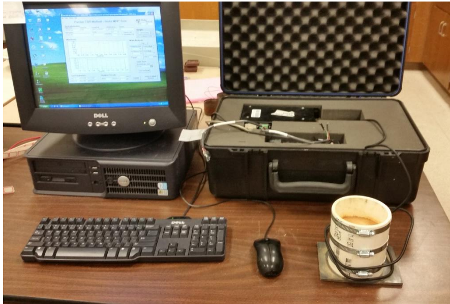
Figure 13. Test setup for evaluation of the suction-TDR sensor performance in silty sand
