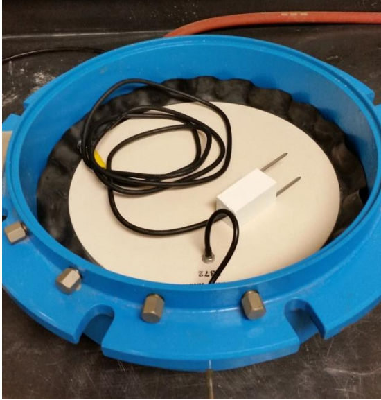
Figure 11. A suction-TDR inside a pressure plate chamber for calibration of suction measurement
