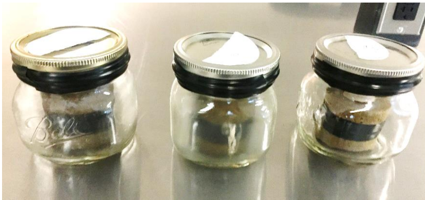
Figure 8. Soil specimens inside a sealed jar for moisture equilibration
