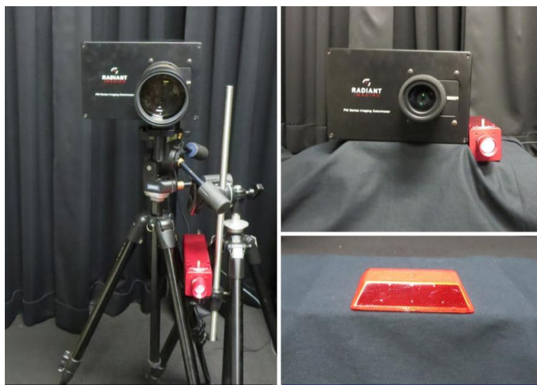
Figure 2-12. CCD photometer data collection setup [2].
