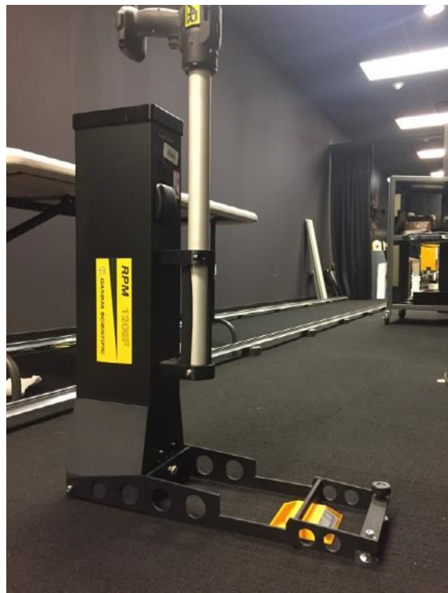
Figure 2-13. Portable reflectometer setup [2].
