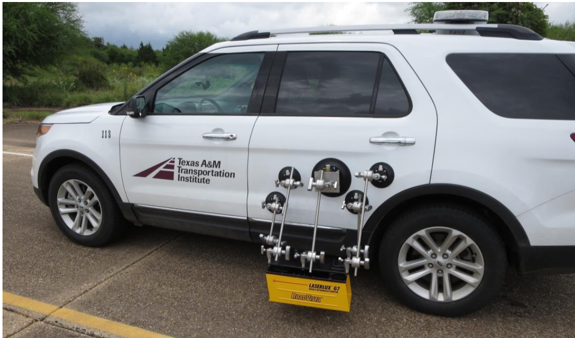
Figure 2-14. Laserlux G7 MRU setup [3].
