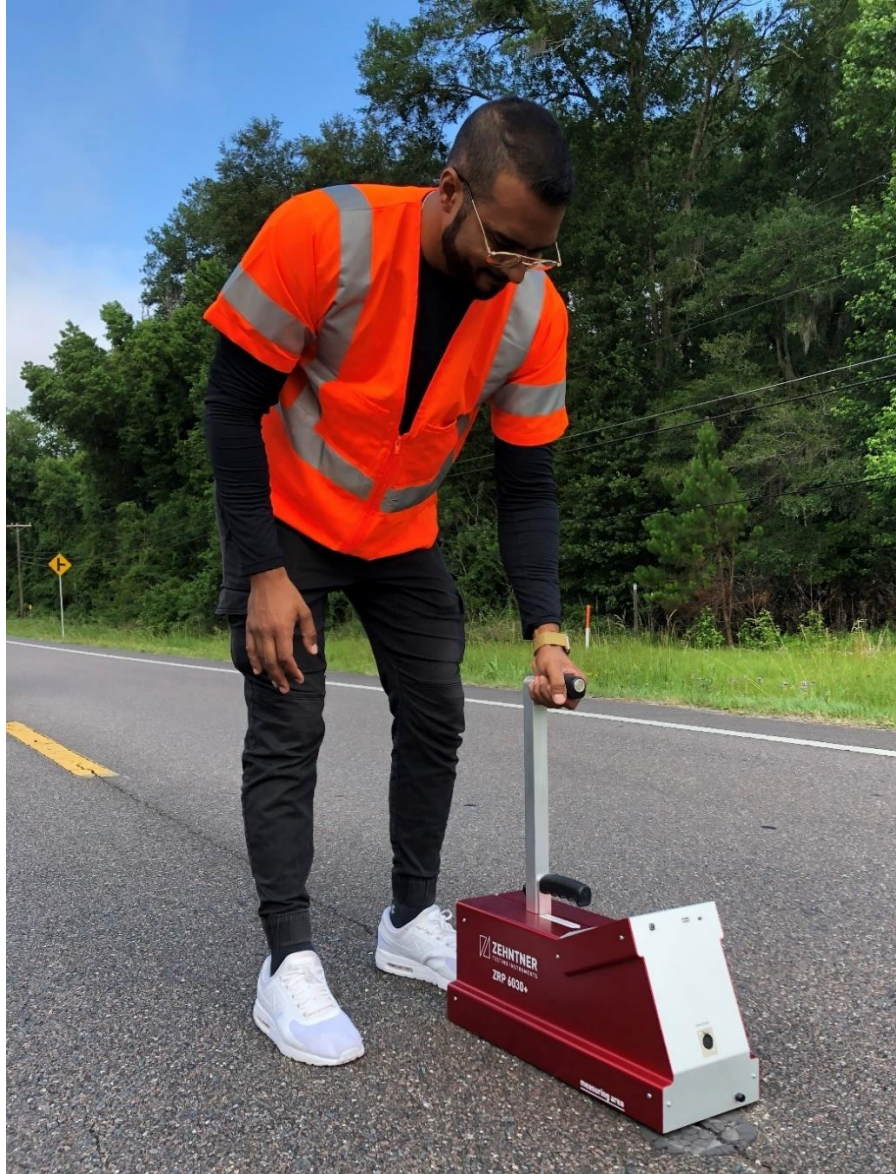
Figure 5-2. Collecting reference data with the Zehntner handheld device.
