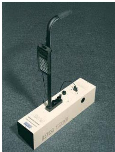
Figure 2-8. Gamma Scientific 1200SP RPM portable reflectometer [1].
