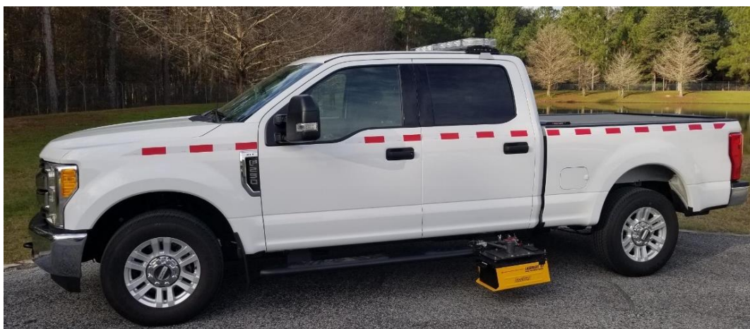
Figure 3-12. FDOT G7 MRU and the test vehicle.
