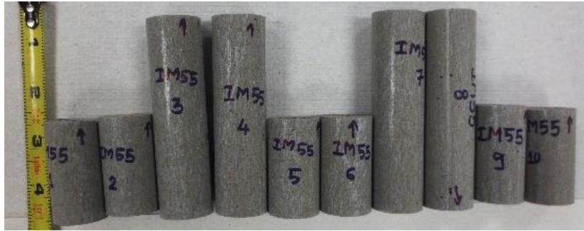
Figure 4.6. INT Test specimen fabrication.
