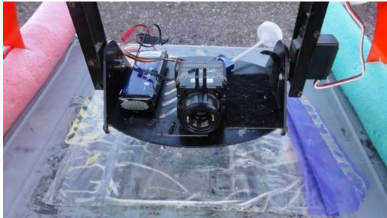
Figure 4.9: FLIR Vue Pro onboard the Bergen Hexacopter
