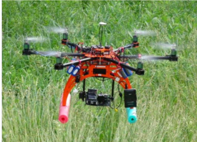
Figure 4.8: MDOT's Bergen Hexacopter with dual FLIR cameras
