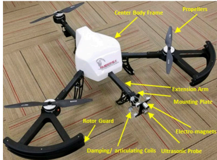
Figure 4.22: Amerapex drone with UT equipment
