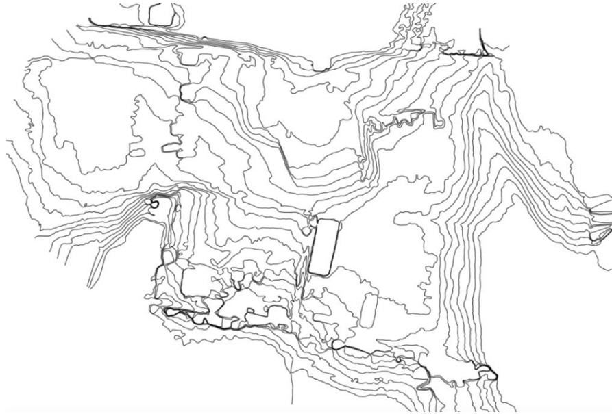
Figure 4.5: Contour map using data collected by a UAV
