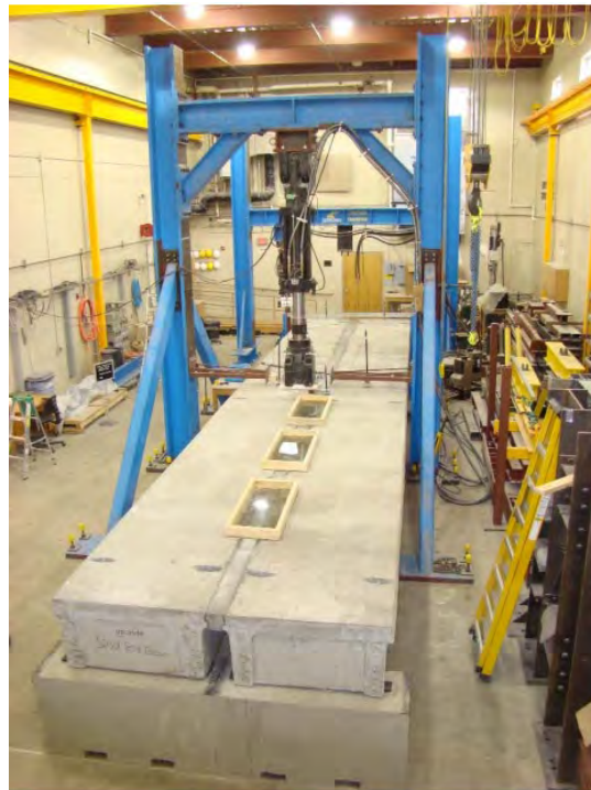
Figure 2.3 Full-Scale Conventional Double-Tee Girder Test Specimen (Konrad, 2014)
