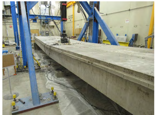
d. Bridge Condition at Failure
