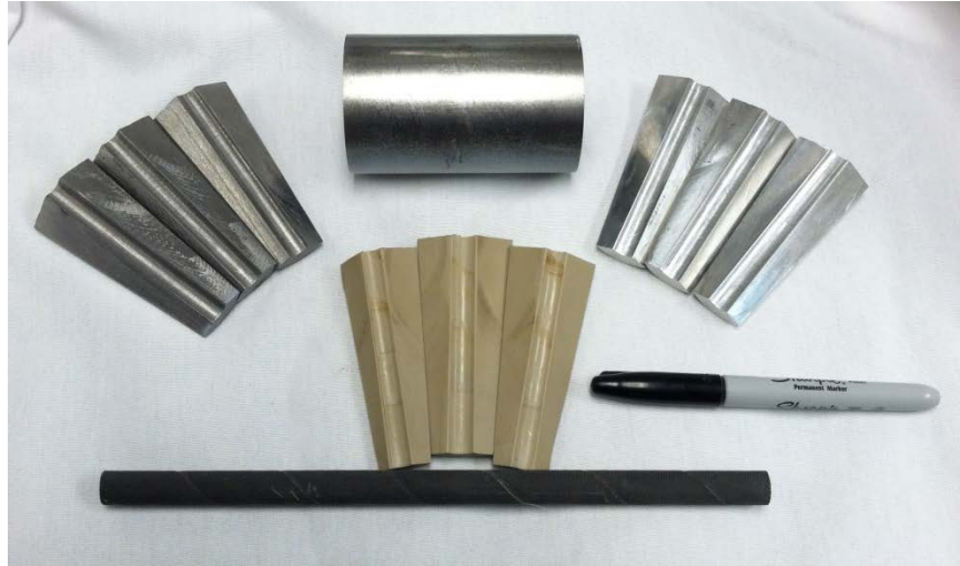
Figure 24. Anchor Prototypes for Straight CFRP Tendons. CFRP = carbon fiber reinforced polymer.
